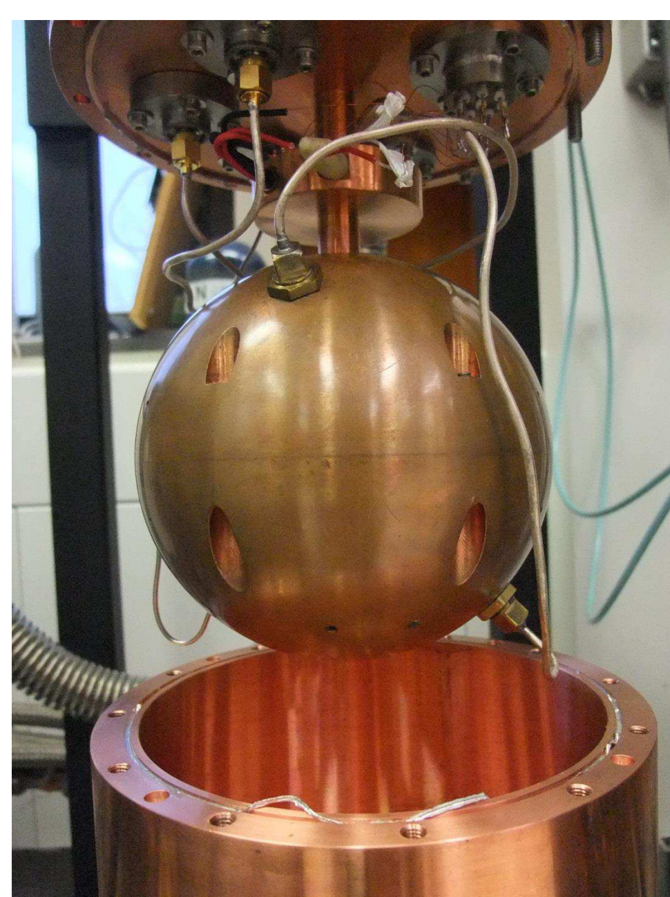
Figure 1. Quasi-spherical microwave resonator & gas pressure vessel From Rourke (2014) [1]
