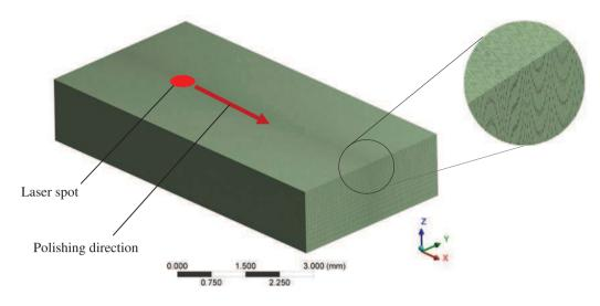
Fig. 1. Meshed geometry of the workpiece.
