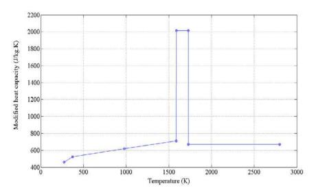
Fig. 2. Temperature-dependent correction of H13 heat capacity
