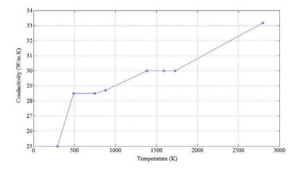
Fig. 3. Temperature-dependent conductivity of H13
