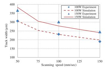
Fig. 9. Simulation and experiment results for steady track width
