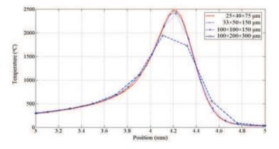
Fig. 8. Mid-track temperature at t = 45 ms
