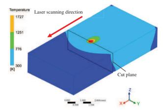
Fig. 5. Sample temperature field 45 ms after the start of the laser beam motion
