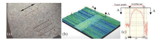
Fig. 7. (a) Representative LPed lines made at 100 W and 150 W; (b) surface topography of a LPed line; (c) LPed line cross-section
