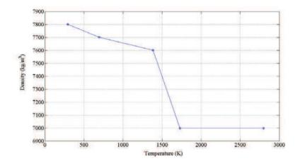
Fig. 4. Temperature-dependent density of H13
