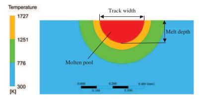
Fig. 6. Sample molten pool geometry as seen in a transversal cut plane
