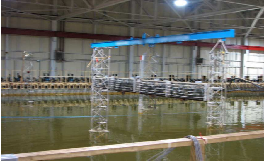
Figure 3.8: Wind fans mounted in the Offshore Engineering Basin.
