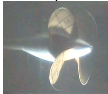
Figure A-2. Photographs showing back cavitation for -15° Puller Propeller at different cavitating conditions.
