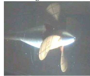
Figure A-2. Photographs showing back cavitation for -15° Puller Propeller at different cavitating conditions.
