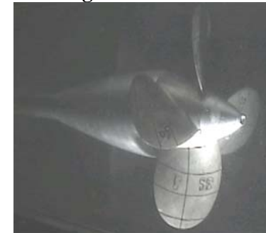
Figure A-4. Photographs showing back cavitation for -20° Puller Propeller at different cavitating conditions.
