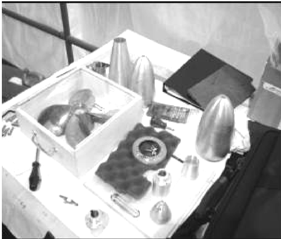
Figure 3-2. Pictures of nose and rear cone adapters for the propellers.
