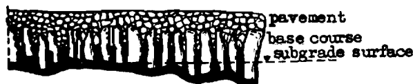
Fig. 3. Actual appearance of pavement and subgrade surface after rolling and under traffic, with a frost-susceptible subgrade. Non-uniform subgrade surface and highly compressed subgrade hamper drainage.
