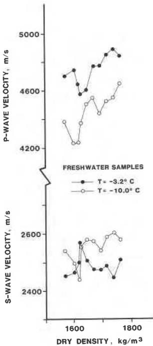
Fig. 1. Effect of changing dry density on acoustic velocities
