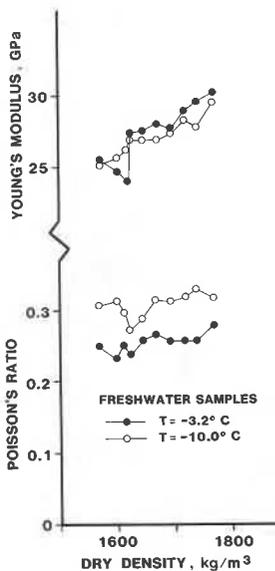
Fig. 2. Effect of changing dry density on Poisson's ratio and Young's modulus
