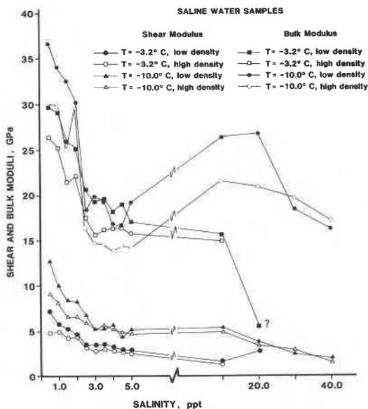
Fig. 8. Effect of changing salinity on shear and bulk moduli
