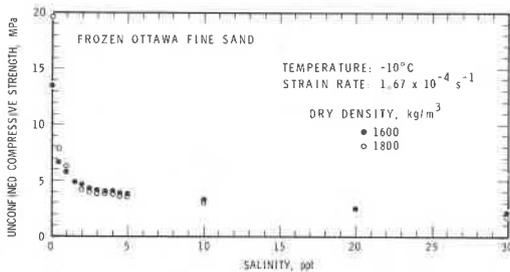
Fig. 10. Effect of changing salinity and dry density on unconfined compressive strength
