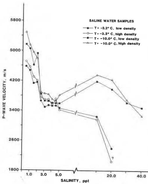
Fig. 4. Effect of changing salinity on compressional wave velocity
