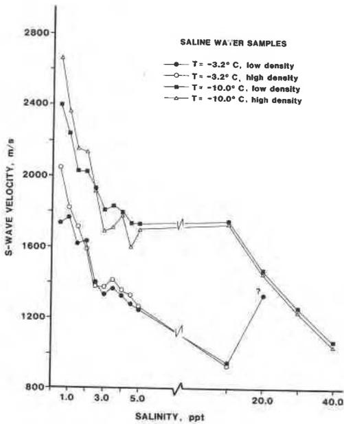
Fig. 5. Effect of changing salinity on shear wave velocity
