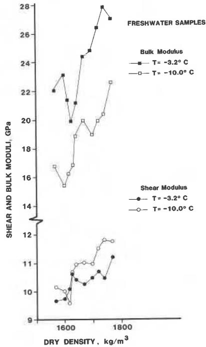
Fig. 3. Effect of changing dry density on shear and bulk moduli
