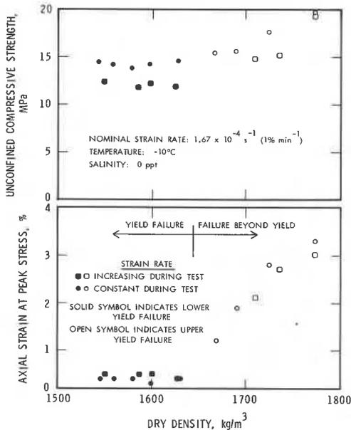
Fig. 9. Effect of changing dry density on unconfined compressive strength and failure strain
