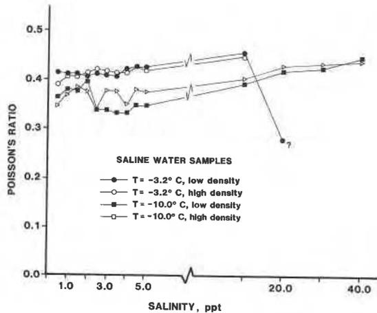
Fig. 7. Effect of changing salinity on Poisson's ratio
