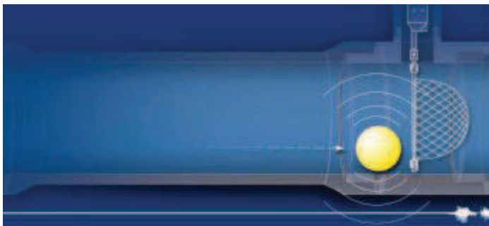
Figure 2. Schematic of an in-pipe leak detection method (Used with permission, Pure Technologies Ltd.)
