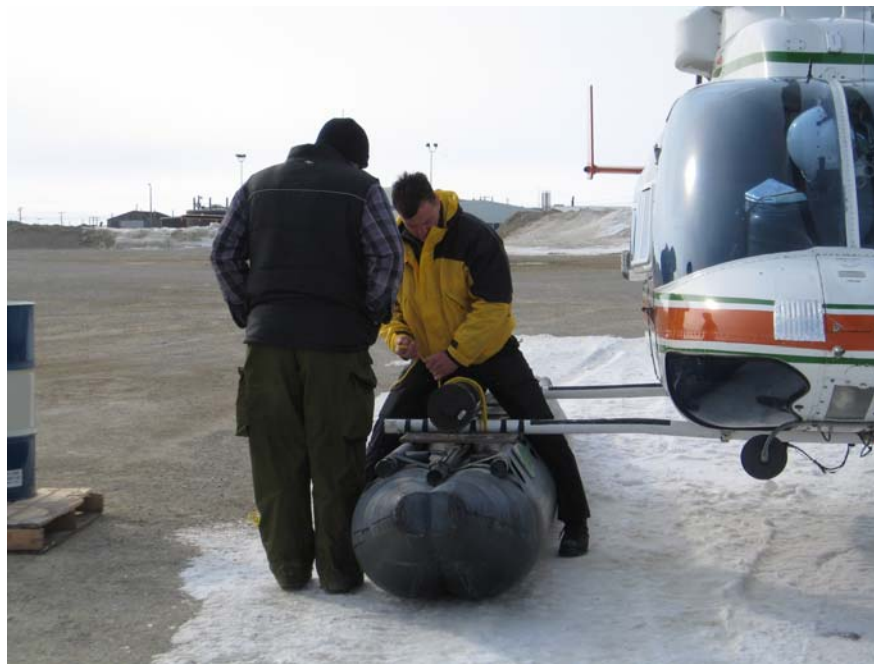
Figure 3 Transporting temperature chain to Floe R02. The five 2 m lengths of temperature chain were sealed in a black ABS tube and securely strapped to the helicopter skids.
