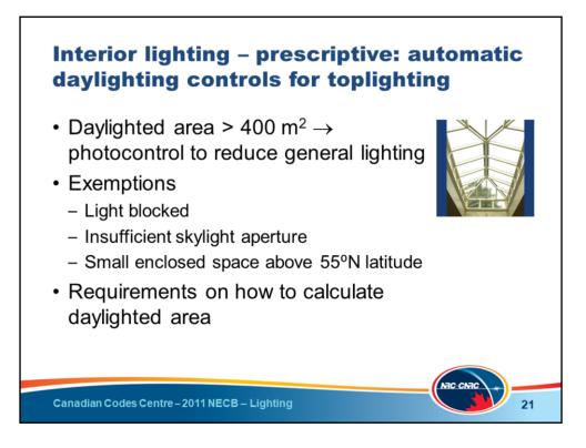
There are requirements for automatic daylighting controls for toplighting (skylights and rooftop monitors).
