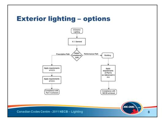
Here you see a flow chart showing the compliance options for exterior lighting. Compliance is achieved using the prescriptive path or through whole-building modeling using the performance path.
