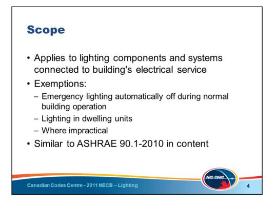
The scope of NECB Part 4 includes lighting components and systems that are connected to the building's electrical service.
