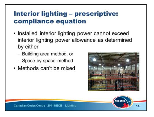
The basic principle of the prescriptive requirements for interior lighting is that the actual installed interior lighting power cannot exceed the allowance for the interior lighting power when the allowance is calculated using either the building area method or the space-by-space method.
