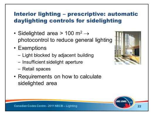
There are also requirements for automatic daylighting controls for sidelighting (windows).
