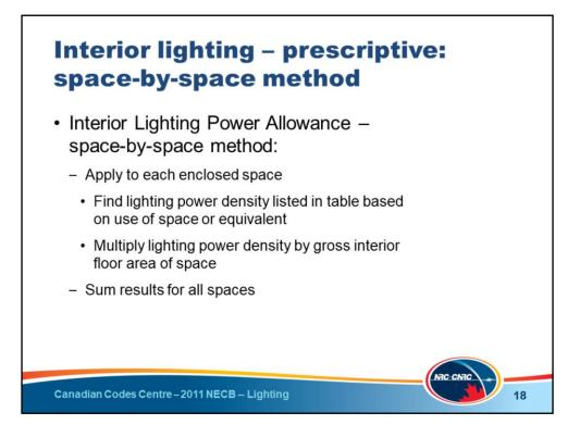
To determine the interior lighting power allowance using the space-by-space method, the lighting power density for each space use, or its equivalent, is determined from a values table. The lighting power density is then multiplied by the gross interior floor area of the space.
