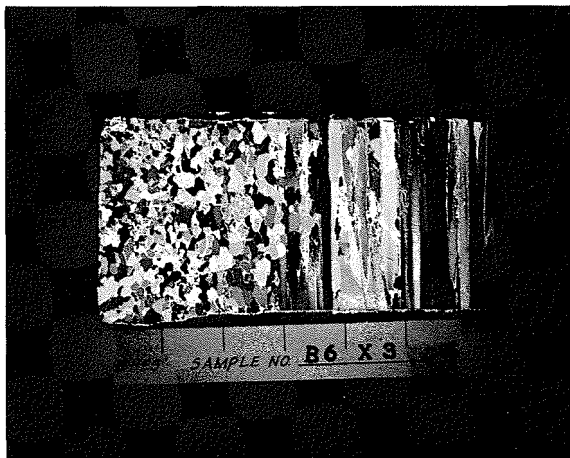
Fig. 7b. Thin Section of Block 6 Cut Perpendicular to the Area of Application of the Load and the Face of the Block. Note the Break-up of the Columnar-Grain Structure that has Occurred Beneath the Area of Application of the Load.
