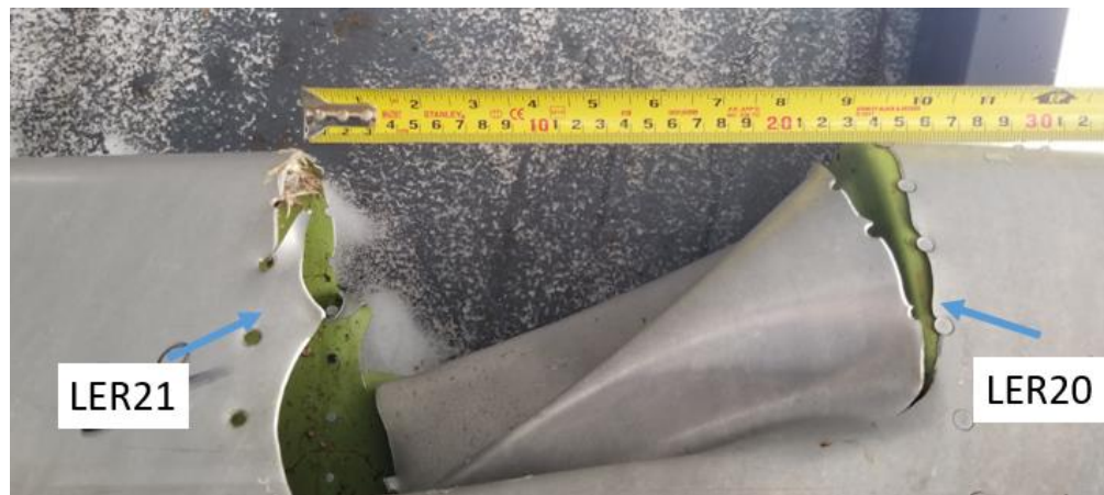
Figure 55: Damage length on the leading edge (HS-T6)
