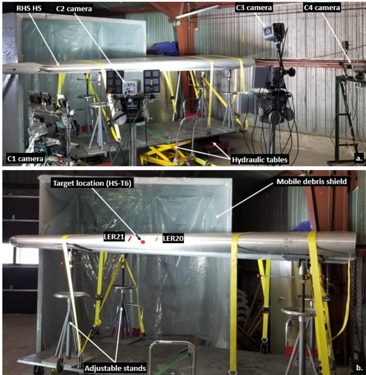
Figure 53: Bird impact test configuration (HS-T6)
