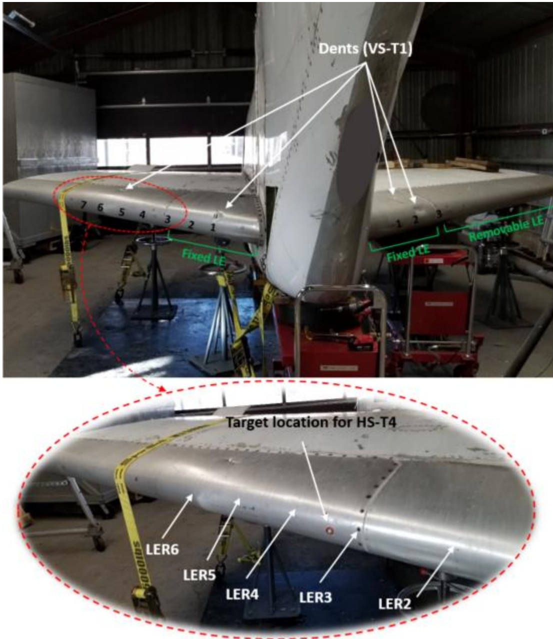
Figure 29: Test setup (HS-T4)
