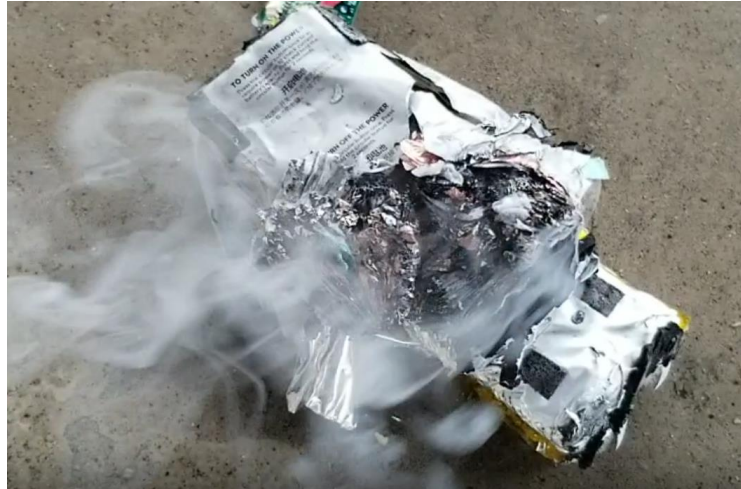
Figure 15: Status of the drone battery after impact
