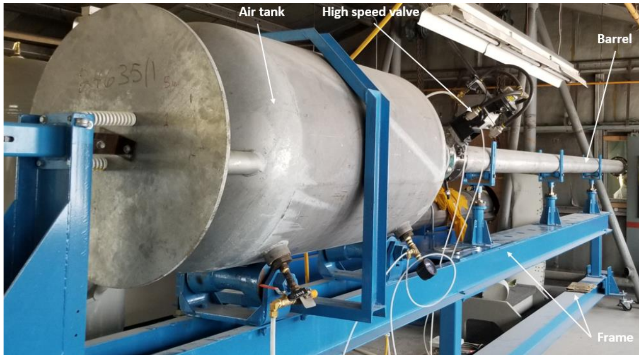
Figure 52: Pneumatic cannon for bird impact (HS-T6)
