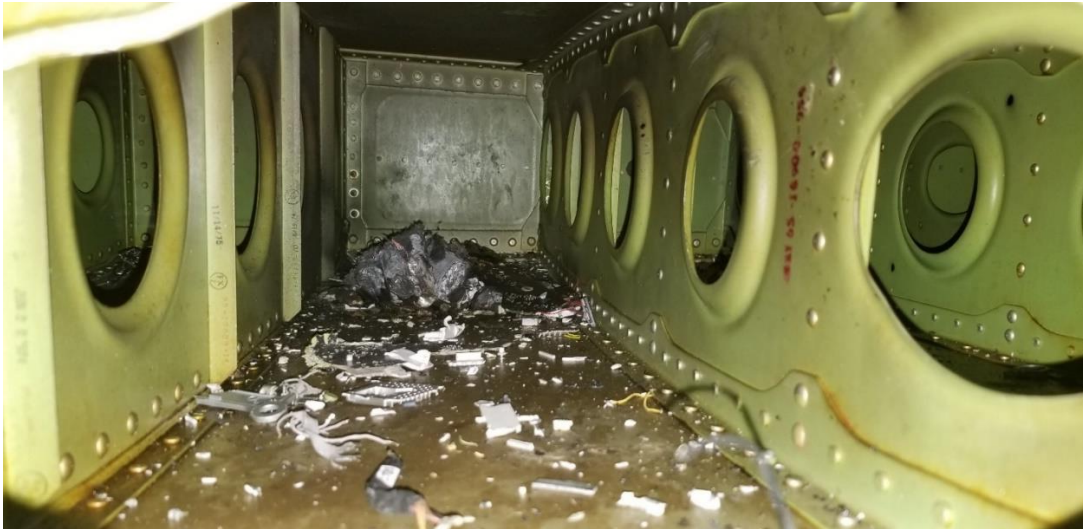
Figure 28: Shattered drone structure and burnt battery debris (HS-T3)
