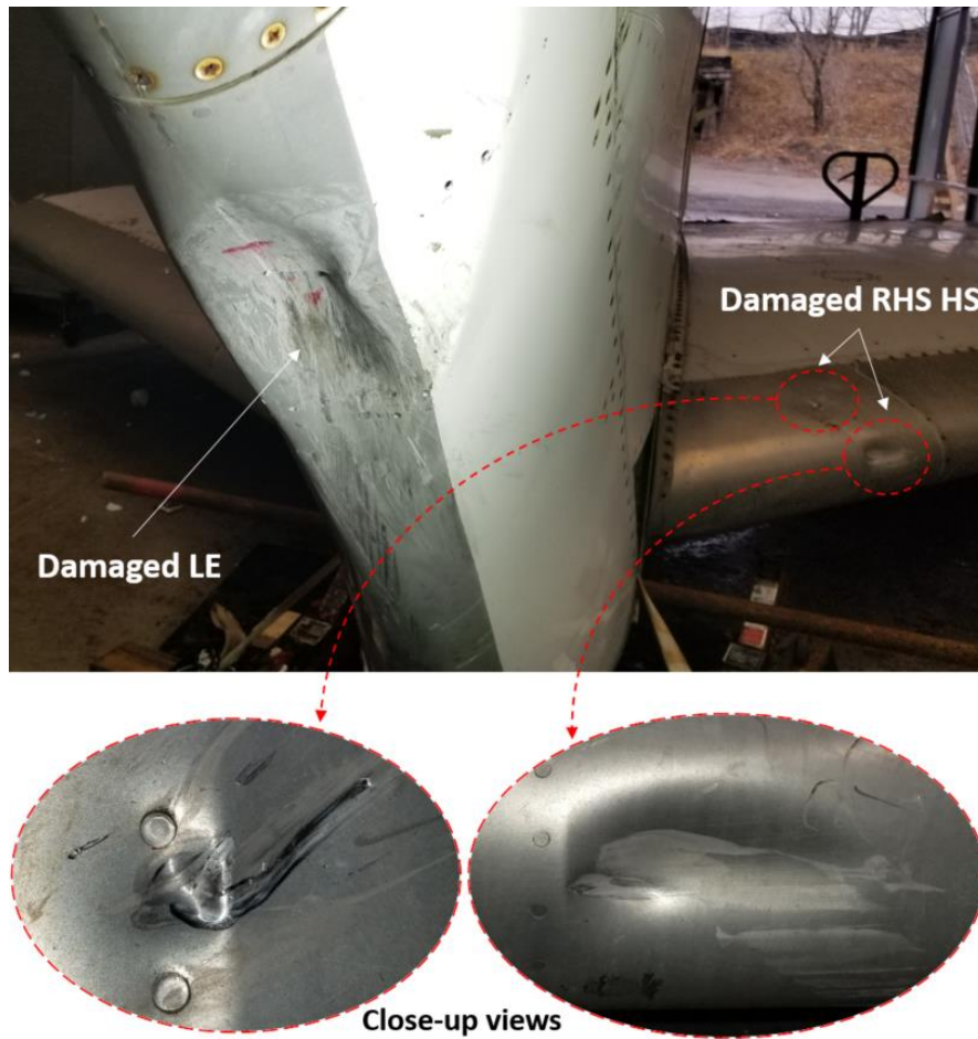
Figure 48: Collateral damage on RHS HS (VS-T1)
