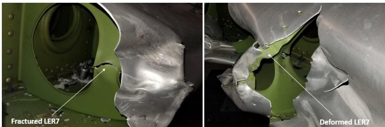
Figure 40: Damage caused to LER7 and its vicinity (HS-T5)
