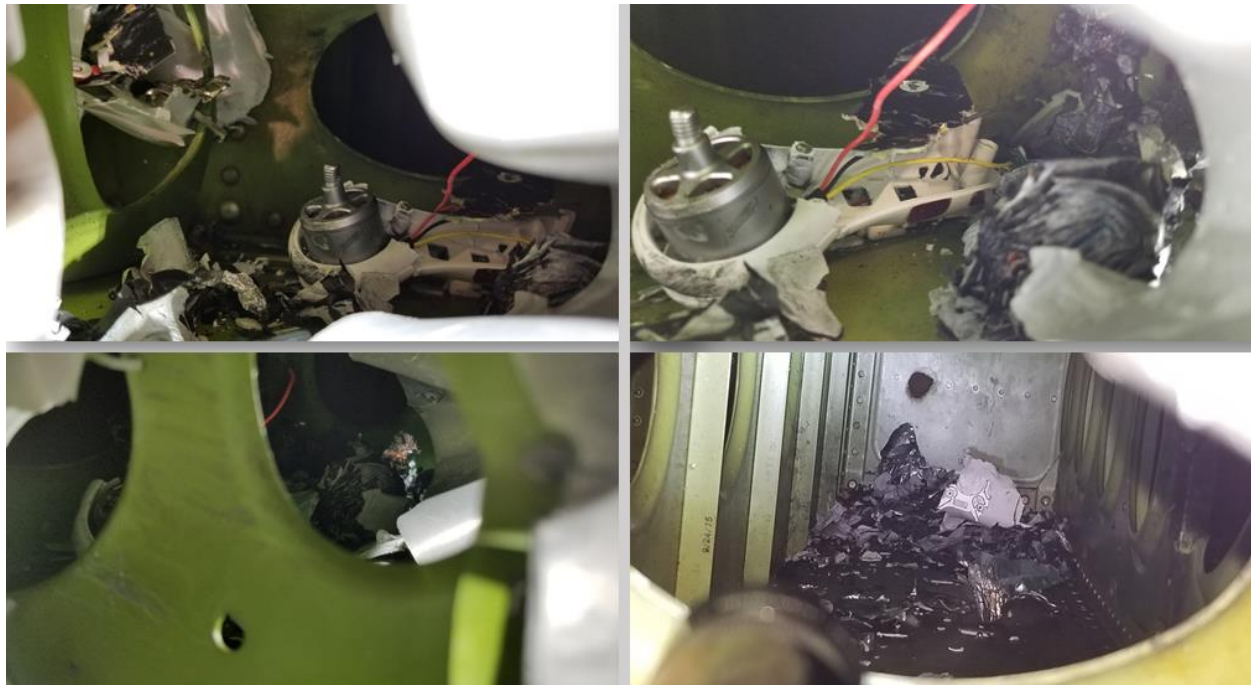
Figure 20: Remains of the test drone inside the HS (HS-T2)
