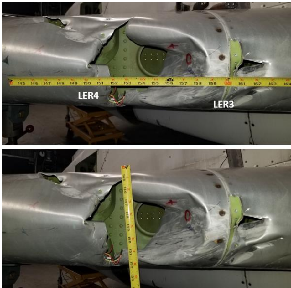
Figure 31: Damage to the leading edge structure (HS-T4)
