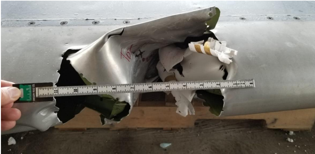
Figure 26: Damage dimension (HS-T3)
