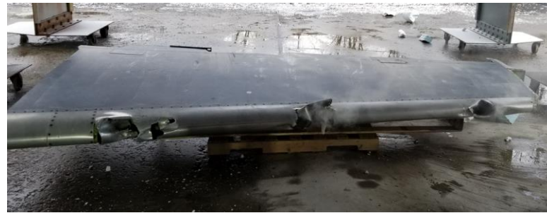
Figure 24: Test segment after impact
