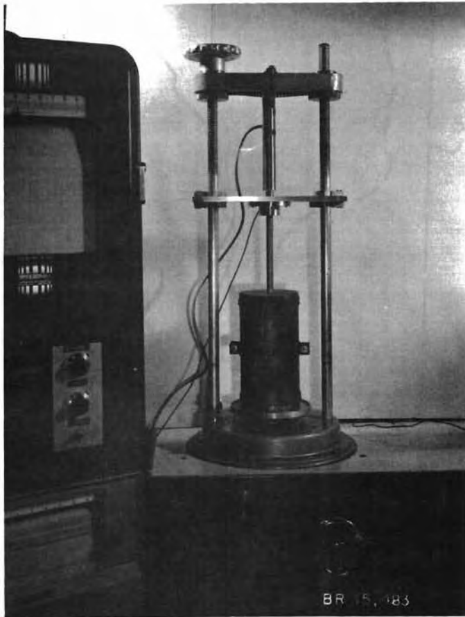
Figure 3: General view of the laboratory penetration test equipment.
