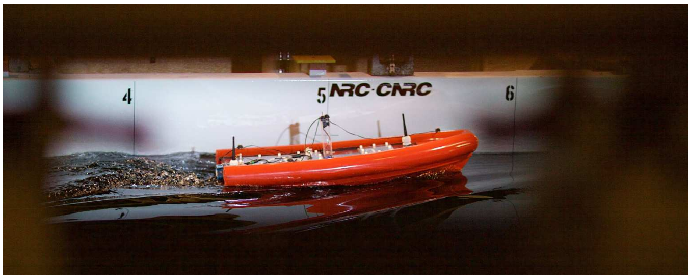
Figure 16 Photos of interactive seakeeping tests in following seas
