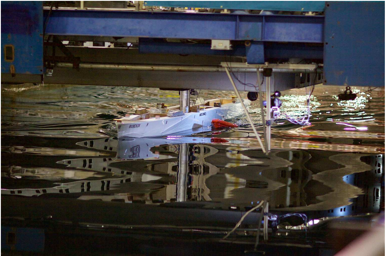
Figure 14 Photos of interactive seakeeping tests in head seas, cont.
