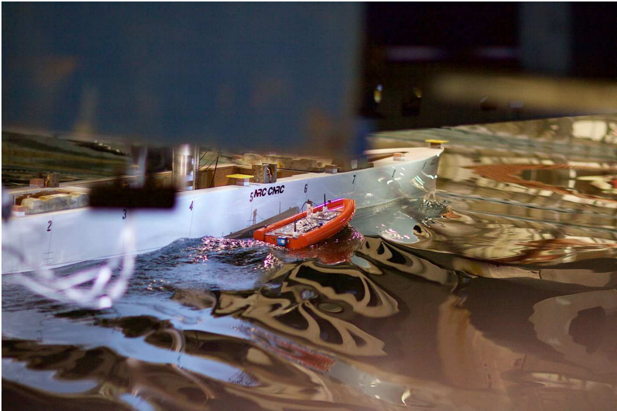
Figure 17 Photos of interactive seakeeping tests in following seas, cont.
