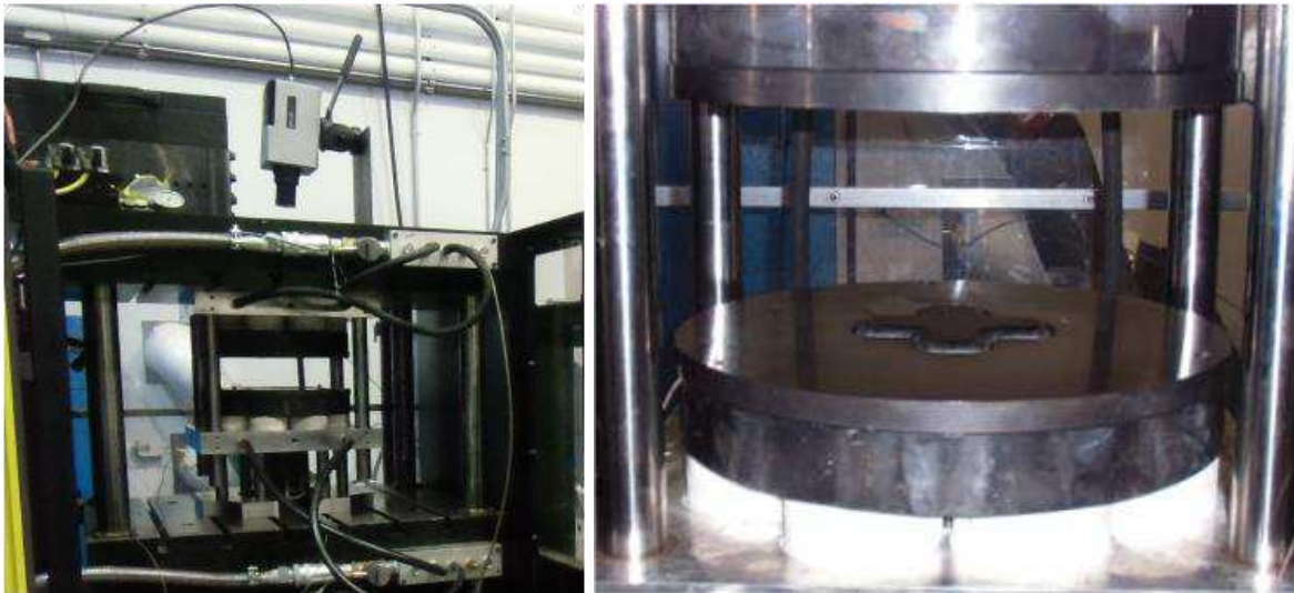
Figure 1. Cross die test setup developed for hot stamping with blank temperature measurements
