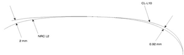
**Figure 5:** A comparison of the new CL-L10 and previous NRC-L2 rail templates.
