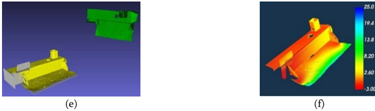
Figure 5. (a) Mesh model with 2 mm resolution of vector field. (b) Mesh model with 1 mm resolution of vector field. (c) CAD model with selected alignment points (d) Scan with selected alignment points. (e) Final alignment of the scan (yellow) on the CAD model (grey). (f) Heat map of distance between scan and CAD model.
