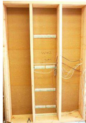
**Figure 13 – W2: Response of moisture detection strip to the presence of moisture in the wall**
