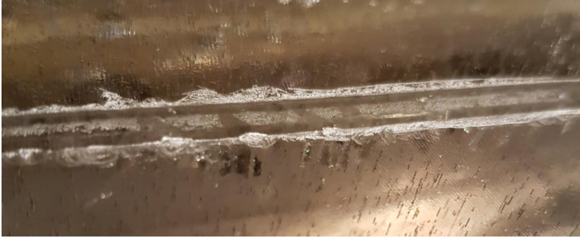
Figure 10. Thin ( < 0.1 mm) white sheet of wispy material sticking up from the ice surface along the sides of the glide track left after a number of tests. The material is the fully-frozen remnant of the thin slurry layer (originally 18 % liquid) that was squeezed out of the forward bow region of the blade during the test. The reader may expand the view on-screen to see fine details. Note that some slurry was also squeezed into the central area of the track where the hollow of the blade provided a small gap (as in Figure 7) between the ice surface and the blade.
