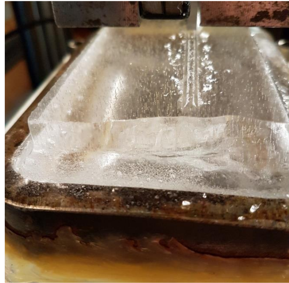
Figure 2. Blade track left following a number of gliding tests. Note that the vertical load is borne on the symmetric contacting portions of the blade's edges. The thin white wispy material is frozen extruded slurry (discussed below).
