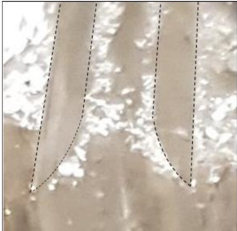
Figure 11. Bow portion of the blade track created by a number of glide tests. The two parallel, but separated, segments of the track (outlined) stem from the ‘hollow’ shown in the sectional profile of the blade (Figure 7). The ‘pointy’ regions on the ends of the segments are due to the upturn of the blade bow. The white material is the fully-frozen remnant of the slurry (~ 18 % liquid by weight) ejected at the bow during gliding. All ice that is removed from the track leaves in the form of slurry.
