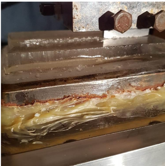
Figure 1. Mock ice-skating blade gliding from left to right on a columnar-grained freshwater ice sample.
