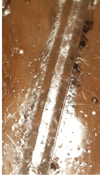
Figure 12. Glide track produced by a number of tests. The wispy fully-frozen slurry (as in Figures 10 and 11) has been swept away to reveal the smooth glide track that shows no signs of plastic deformation or mounds of refrozen melt at the sides or center.
