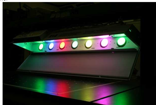
Figure 2. Custom luminaire. Left photo: exterior of troffer (shown suspended from lab bench). Right photo: LED sources are individually controllable and are aimed at the side of the troffer to provide a diffuse light through the prismatic lens.
