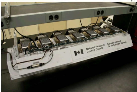
Figure 2. Custom luminaire. Left photo: exterior of troffer (shown suspended from lab bench). Right photo: LED sources are individually controllable and are aimed at the side of the troffer to provide a diffuse light through the prismatic lens.
