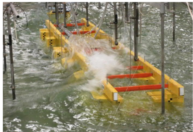
Figure 2 - Wave loads and pressures were measured on a 1/35 scale model of a gravity-based structure.
