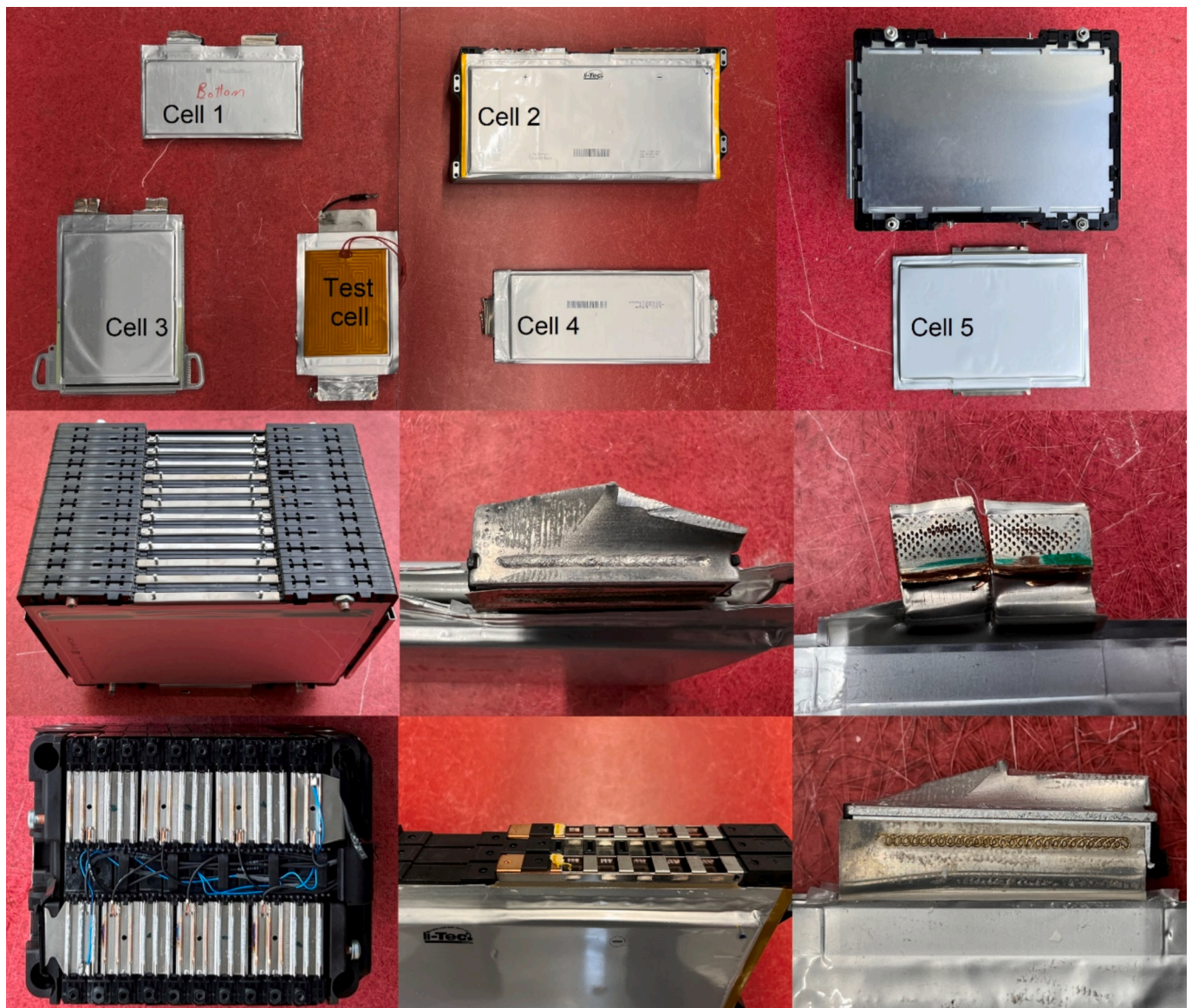
Fig. 9. A photograph of OEM pouch cells and modules used in EVs.
