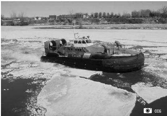
Fig. 14. The CCGS Waban-Aki air cushion vehicle used for icebreaking in the St. Lawrence river.
