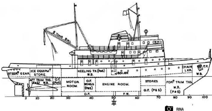
Fig. 10. The *Perkun*, one of the first icebreaker to be model tested (Corlett and Snaith, 1964).
