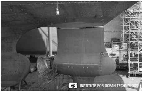
Fig. 24. A typical Azipod installation.
