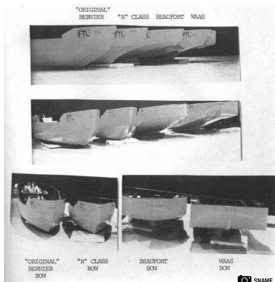
Fig. 21. Models of typical icebreaking bows showing from L-R, the original bow of a CCG Navaid's tender *Bernier*, an R-Class bow, a Beaufort Sea type bow, and a Thyssen-Waas bow (Glen et al. 1998).
