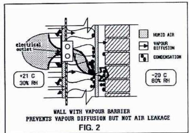
This does not mean that diffusion control is unimportant and that the vapour barrier can be omitted. A vapour barrier is important, particularly in high humidity buildings such as computer centers, museums, hospitals, and public swimming pools.
