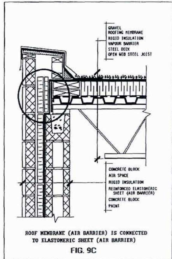
The insulation could be attached to the air barrier (which could also serve as a vapour barrier) followed by an air space and the block veneer. This design change brings a positive solution to the airtightness function of the wall.
