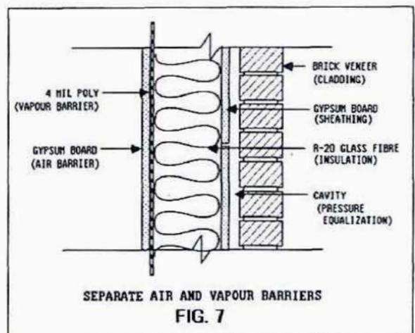
as the polyethylene. The layer of gypsum board sheathing can meet all the requirements of airtightness if all joints are taped and a continuous air seal with other components of the envelope is provided. Although the gypsum board may not be as durable as sheet steel, it is accessible and therefore serviceable.
