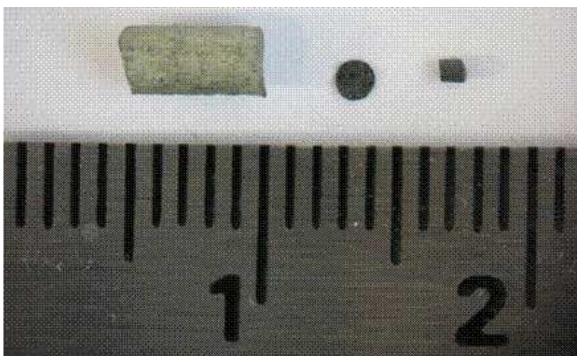
Figure 1. Micrograph of the three propellant formulations. From left to right: SP 7993, SP Unique, and CRM170
