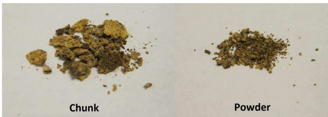
Figure 40. Photograph of the 2-year aged GIM sample after hand mixing
