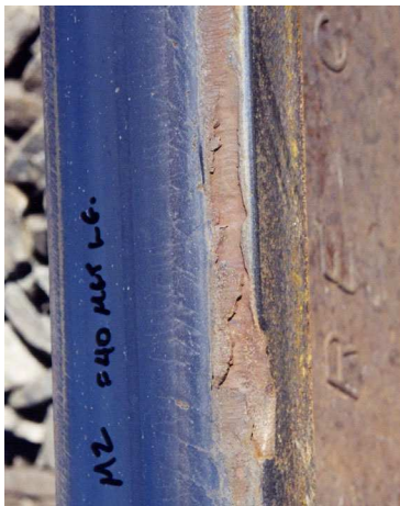
A) gauge corner collapse in a dry environment
