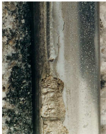
B) gauge corner collapse in a well lubricated rail
