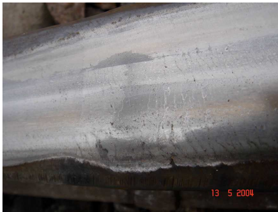
A) High rail, soft weld
