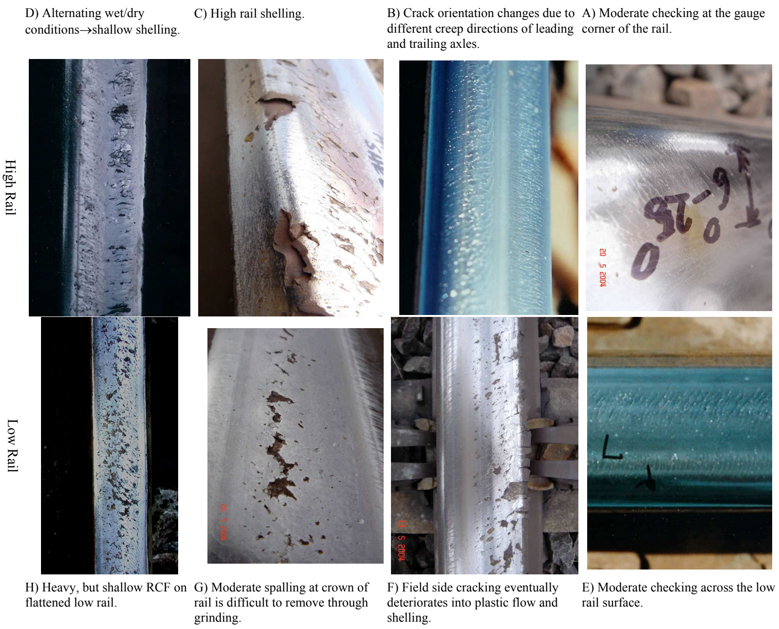
Figure 1: Examples of typical low rail checking and shelling.
