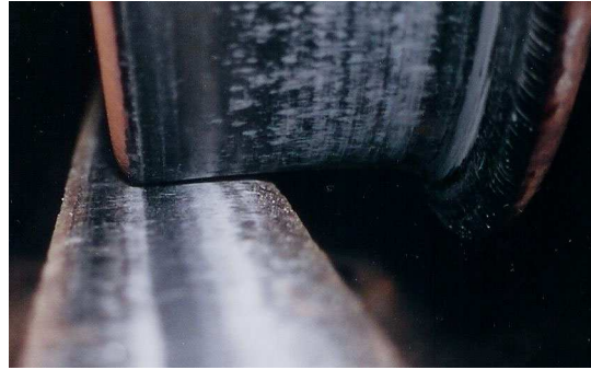
Figure 4: A hollow wheel is especially devastating to wide gauge track where the contact stresses can be very high.
