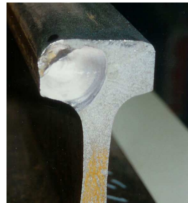
C) transverse defect from a deep-seated shell.
