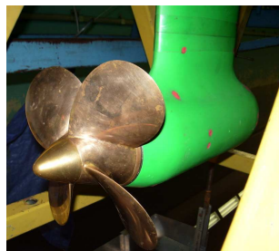
(e) propeller and the pod encasing the pod dynamometer
