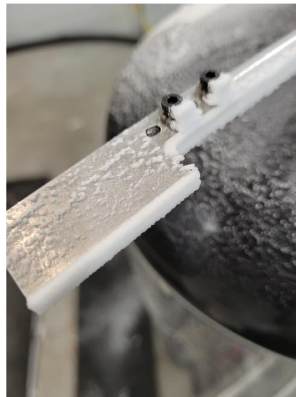
Figure 44: Ice accreted to the leading edge of icing blade
