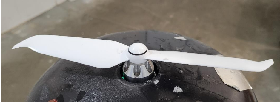
Figure 48: RPAS blade installed on RPAS rotor test rig
