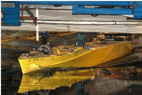
Figure 4: Bare Hull Resistance Test
