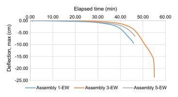
Figure 7. Deflection distributions for exterior wall Assemblies with OSB sheathing and different type of insulations, 1 -EW (GFI), 3-EW (RFI) and 5-EW (CFI) [16].
