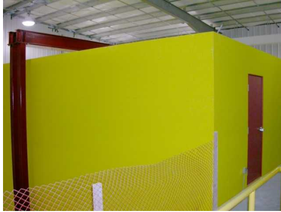
Figure A.3 - 2: Photograph of the NRC\IRC Flanking Transmission Facility showing the loading beam (in red) used to apply the static load to specimen bearing walls.
