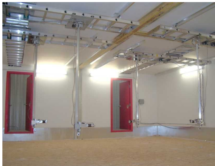
Figure A.3 - 3: Photograph of the NRC Flanking Transmission Facility showing the robots used to position microphones in the upper four rooms. Photo taken before walls of the specimen were installed.
