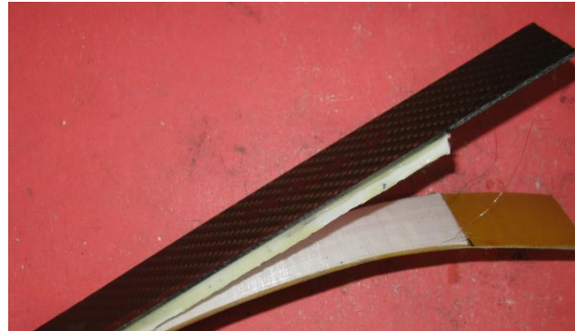
Figure 31: Peel tests showing failure within UHMWPE
