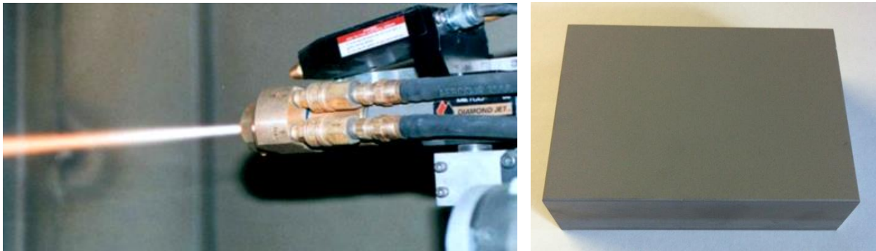
Figure 16: HVOF gun in operation (left) and thick HVOF cermet coating deposited on high-strength Al alloy (right).
