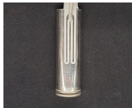
Heating element V4B positioned on a 21700 cell.
