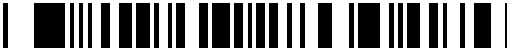
Figure 1: PLIM marker:Marker #0 of the 7-bit family. Pseudo-random binary sequence encoded in a bitonal image. This pattern repeats after 127 bits, typically a minimum threshold ( len_{check} ) of 20-27 bits must been seen at once. Other patterns repeat in longer periods but require a higher minimum threshold.
