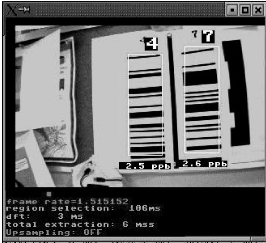
Figure 2: Detection of PLIM markers in image. Fiducial Marker Systems contain both a pattern library and algorithms/software to find them in images. Markers #4 and #7 of the 7-bit family are located in this image. This is a screen shot from a real-time program where each image frame is analyzed for PLIM markers. The markers are assumed to be vertical. The detected region is overlaid with a white box.
