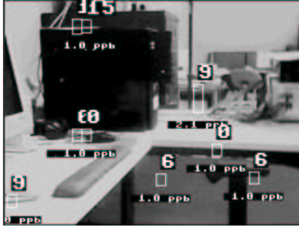
Figure 6: False PLIM markers detected in the image by lowering len_{check} . The len_{check} variable directly determines the upper bound of the probability of falsely reporting a marker when one is not present.
