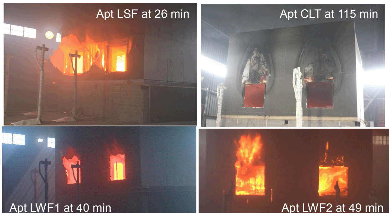
Figure 34. Ventilation conditions through the exterior openings during the large-scale apartment fire tests.
