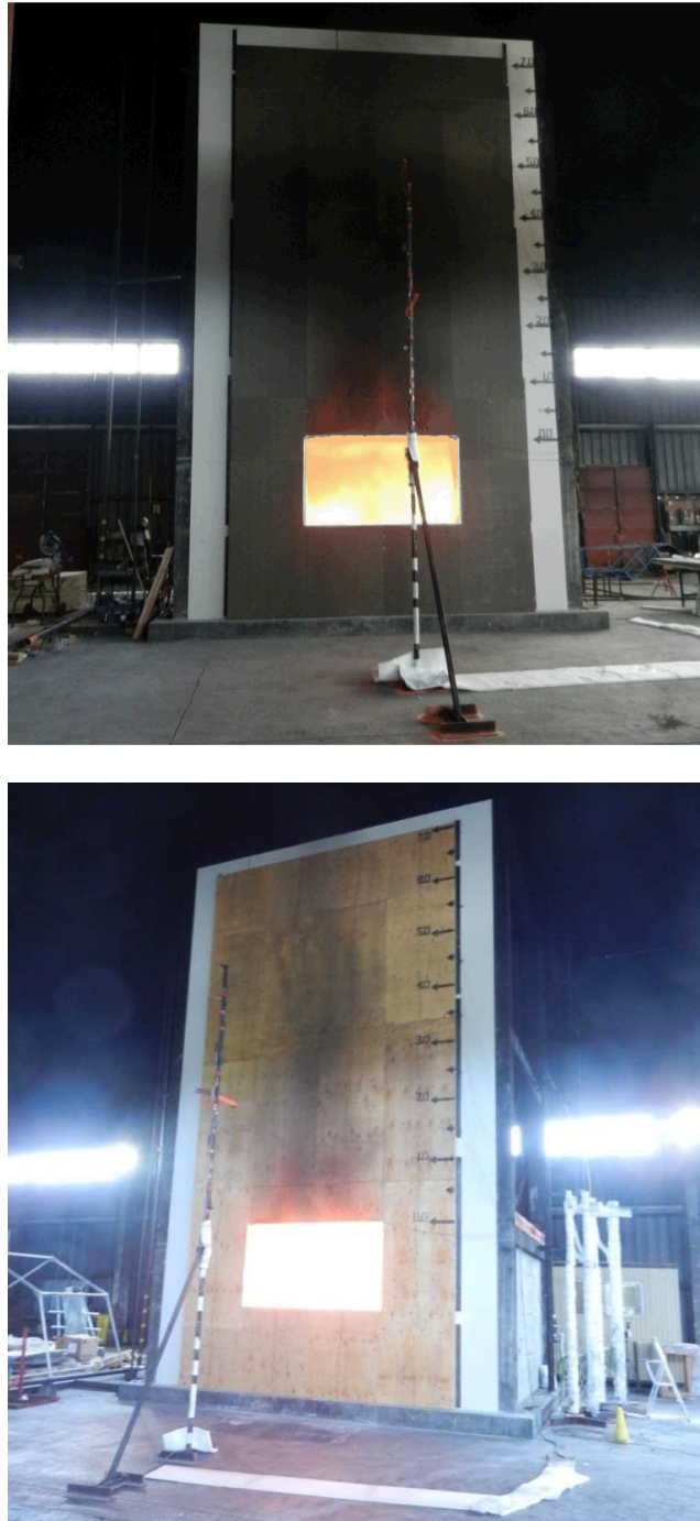
Figure 6. Tests of Exterior Wall Assemblies.
