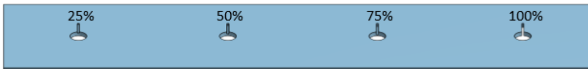
Figure 9: Schematic view of the back side of the specimen showing the three partially penetrating notches and the through-wall notch (right)
