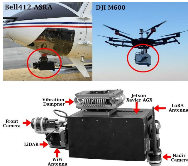
Fig. 1 - The developed multi-sensor payload unit attached to a fixed turret under the nose of Bell 412 Advanced Systems Research Helicopter (ASRA) in NRC-FRL facility is shown in the top-left and top-right shows payload unit attached to a DJI M600 Drone.
