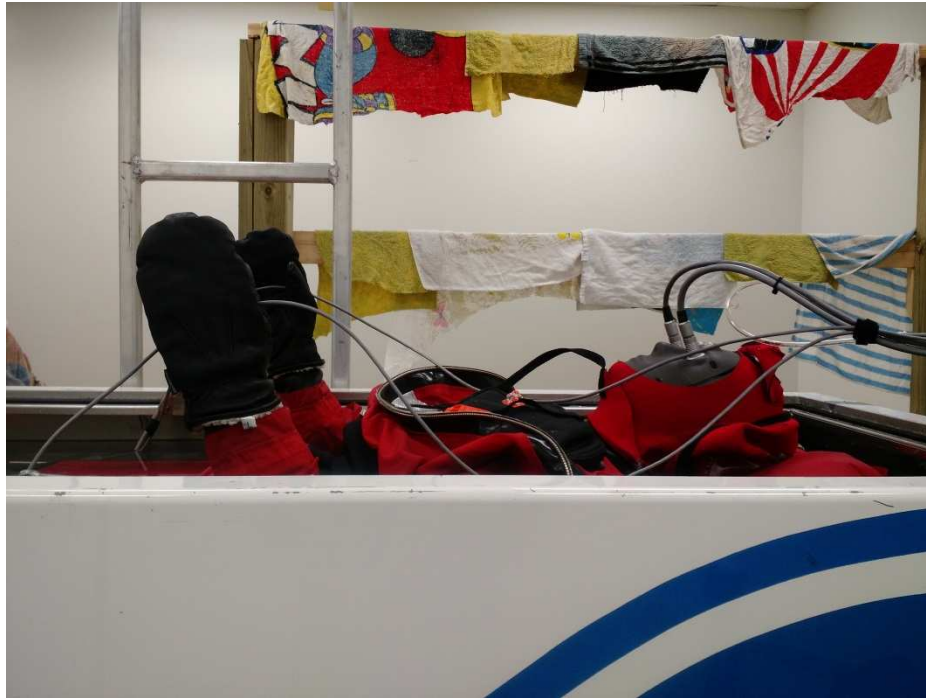
Figure 2. NEMO immersed in the water calorimeter during a typical test.
