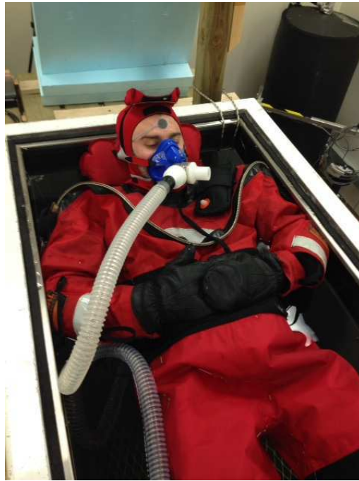
Figure 1. A participant in the water calorimeter during a typical test.
