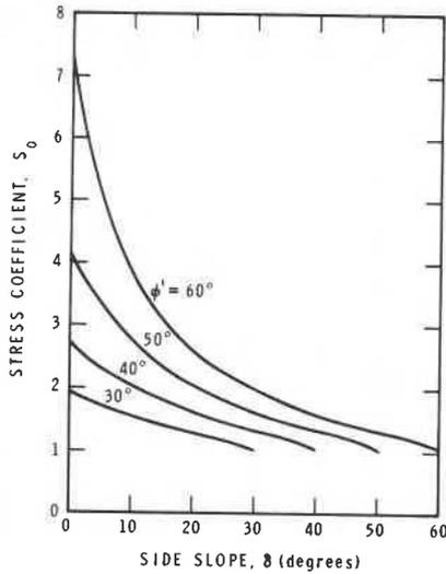
Figure 2 Stress coefficient,  $S_0$ , for symmetrical wedges
