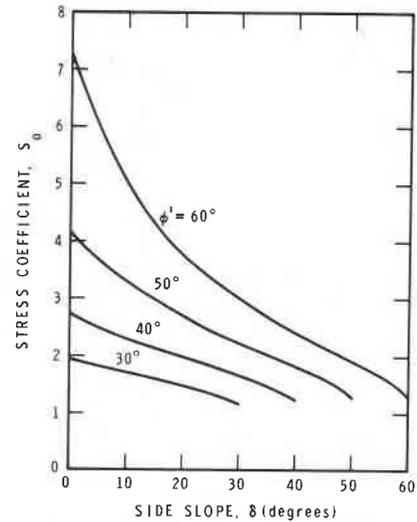
Figure 3 Stress coefficient,  $S_0$ , for asymmetrical wedges with one horizontal side ( $\delta_2 = 0$ )
