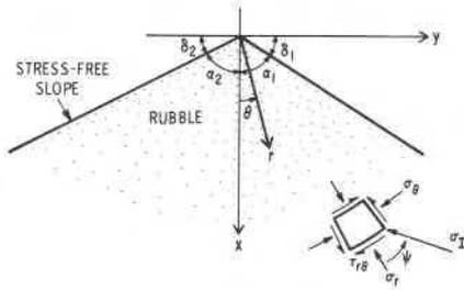
Figure 1 Sketch of two-dimensional wedge
