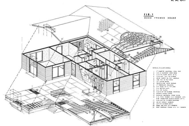
template to assure speed and accuracy. Fixture backing plates, provision for plumbing, heating, etc. (as dictated by the home plan) are built-in to wall sections. Exterior wall studs and plates are precut and assembled on a jig table template in the factory and exterior plywood sheathing is nailed to the stud wall.
