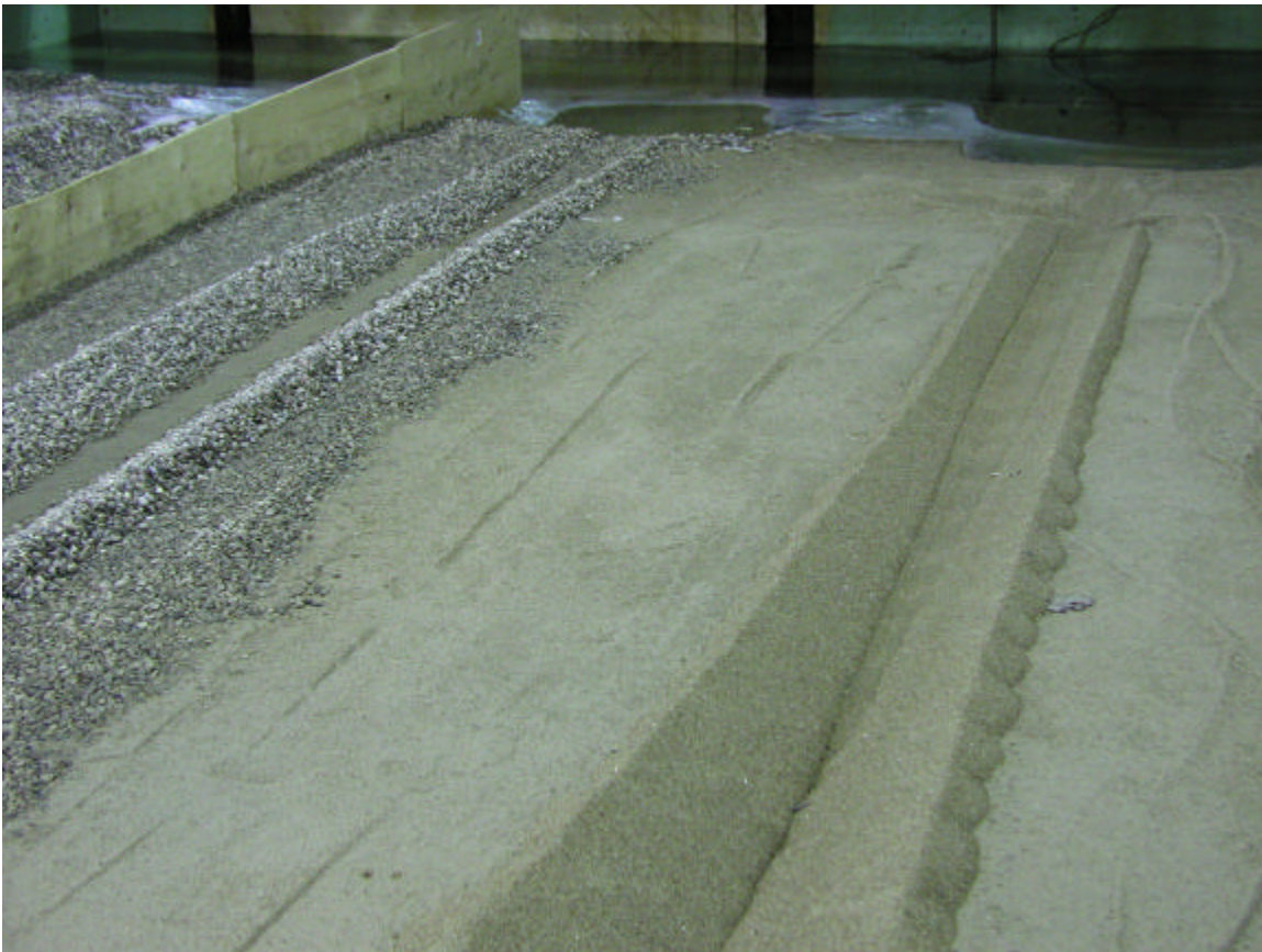
Figure 27 Photograph of two of the drained channels after the second series of three tests.
