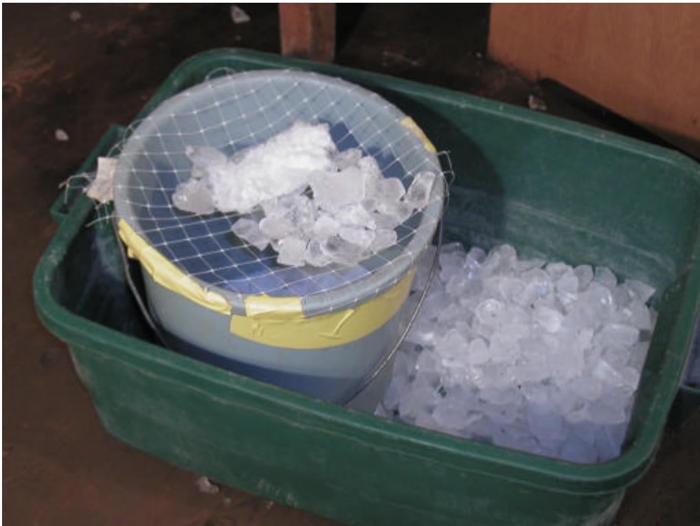
Figure 8 “Filtering” ice for models, through a 0.02 m screen
