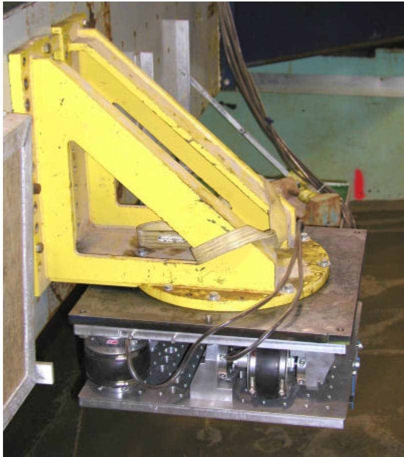
Figure 14 6-component dynamometer underneath mounting bracket and plate
