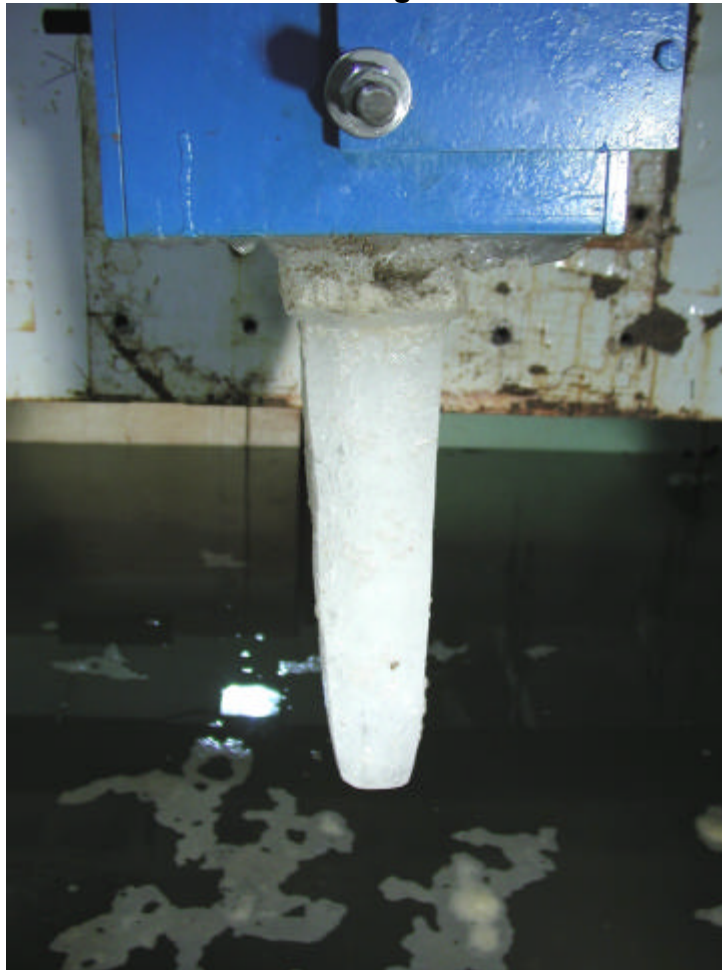
Figure 31 Ice model #3, initially 0.1 m wide over the entire length, before and after testing
