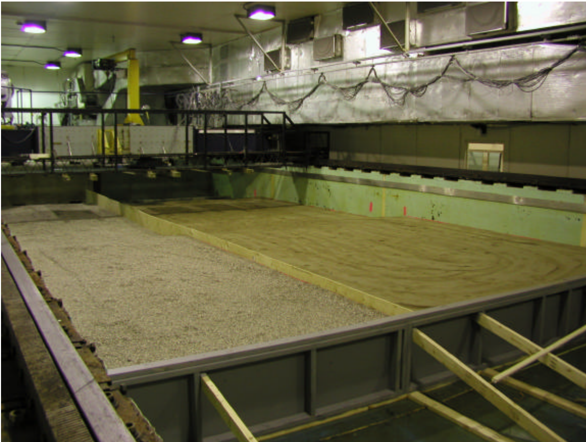
Figure 4 Seabed preparation – gravel on left side, sand on right
