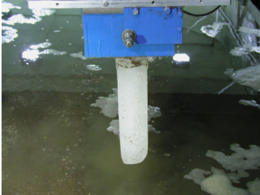
a) 0.1 m ice model before testing
