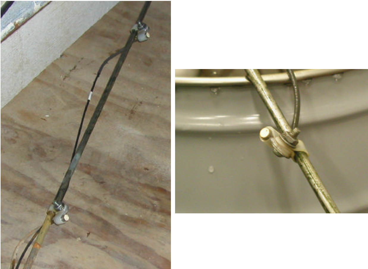
Figure 16 Pore pressure transducers mounted on stainless steel rod
