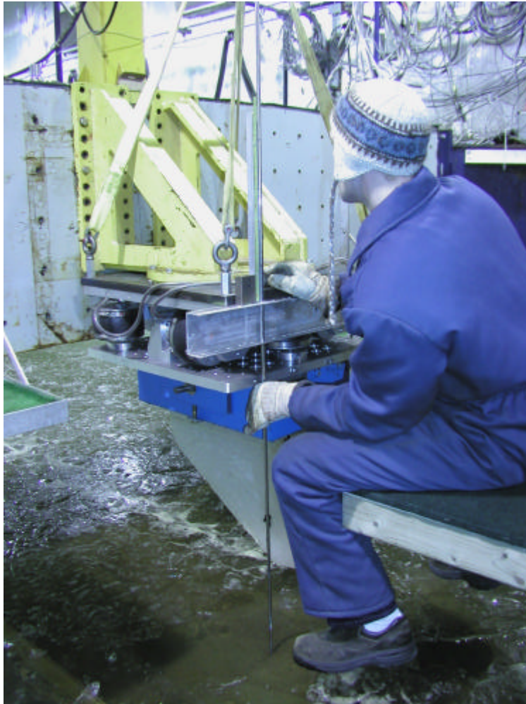
Figure 20 Profiling the scour track
