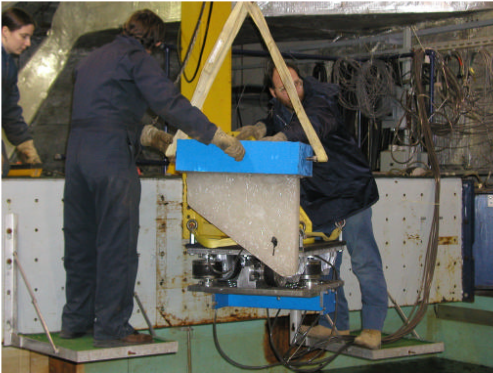
Figure 13 Installing the 0.1 m model below the dynamometer.
