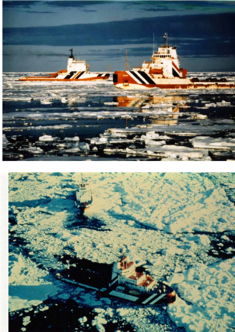
Figure 2.2: CAC 2 icebreakers provided very effective ice management support for the Kulluk. The upper photo shows two of Gulf Canada's icebreakers, the Terry Fox (24,000 HP) in the background, and the Ikaluk (14,800 HP) in the foreground. Their sister ships were the Kalvik and Miscaroo, respectively. The lower photo shows two of these icebreakers fragmenting a very thick and heavily deformed rubble field that was threatening the Kulluk at the time.
