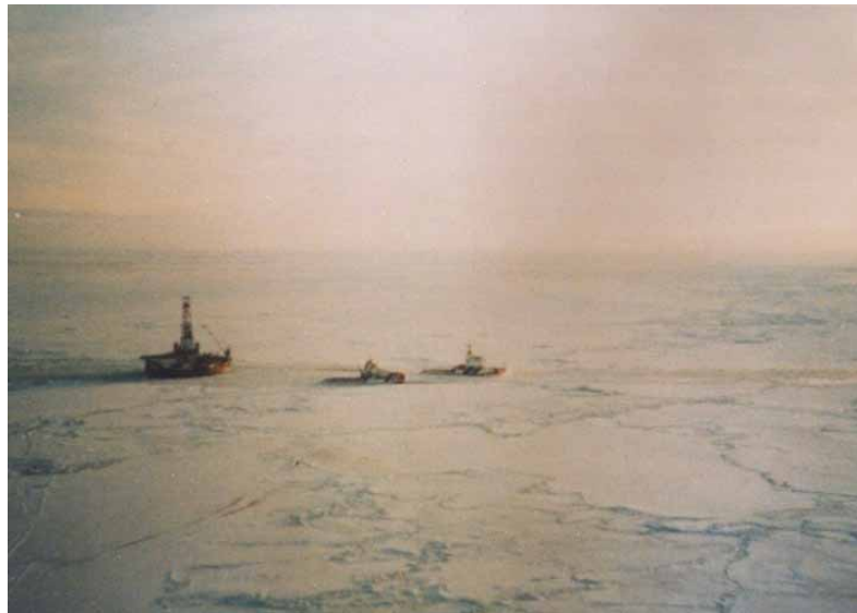
Figure 5.7: An ice management technique that involved high speed icebreaker transits, often in tandem, was used to quickly fragment large “swaths” of pack ice, particularly in fairly thin first year ice conditions. This method is illustrated in the upper part of the figure. After running “up and then back” along the drift line, the icebreakers would stand by the Kulluk for any tactical support that may have been required, thereby saving fuel (lower figure).
