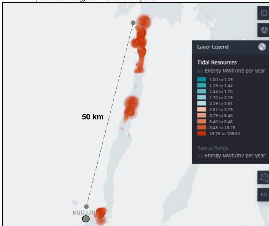
Figure 8: Annual energy near Kuujuaq. There is significant hydrokinetic energy (10-60 MWh/m<sup>2</sup>) along the river near Kuujuaq and towards the river's mouth (50 km away from the community).
