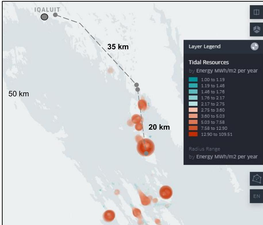
Figure 7: Annual energy density near Iqaluit. Most of the hydrokinetic energy (10-50 MWh/m<sup>2</sup>) is located 50 km from the community between Frobisher Bay Islands. There is limited hydrokinetic energy near the community itself.
