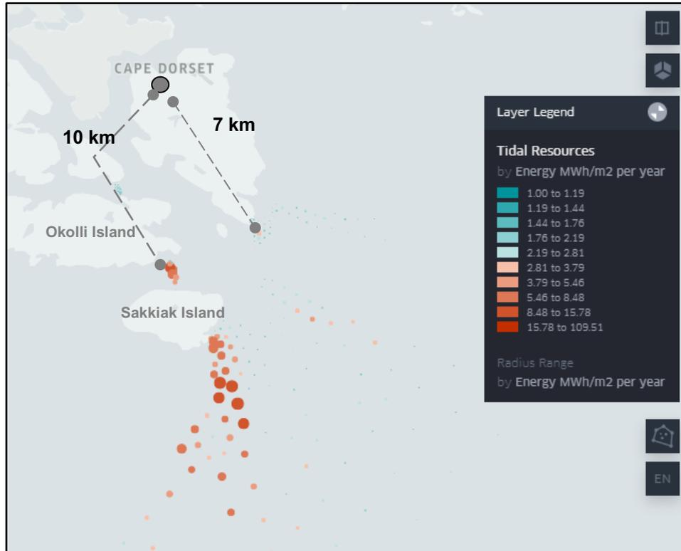
Figure 5: Annual energy density near Cape Dorset. Most of the hydrokinetic energy (5-10 MWh/m<sup>2</sup>) is located on the north and south sides of Sakkiak Island. However, there is some energy (1-2 MWh/m<sup>2</sup>) on the south shore of Dorset Island, approximately 7 km from Cape Dorset.
