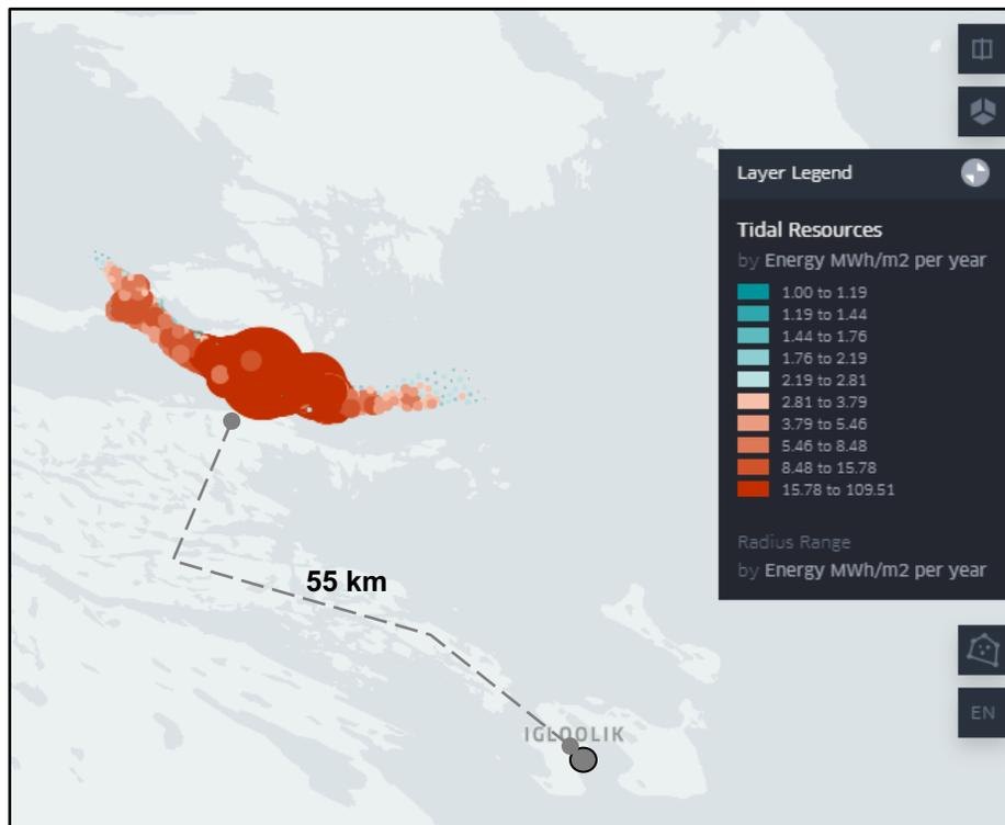
Figure 6: Annual energy density near Igloolik. There is significant hydrokinetic energy (50-100 MWh/m<sup>2</sup>) in the Labrador Narrows, which is 50-60 km from the community. There is limited hydrokinetic energy near the community of Igloolik itself.
