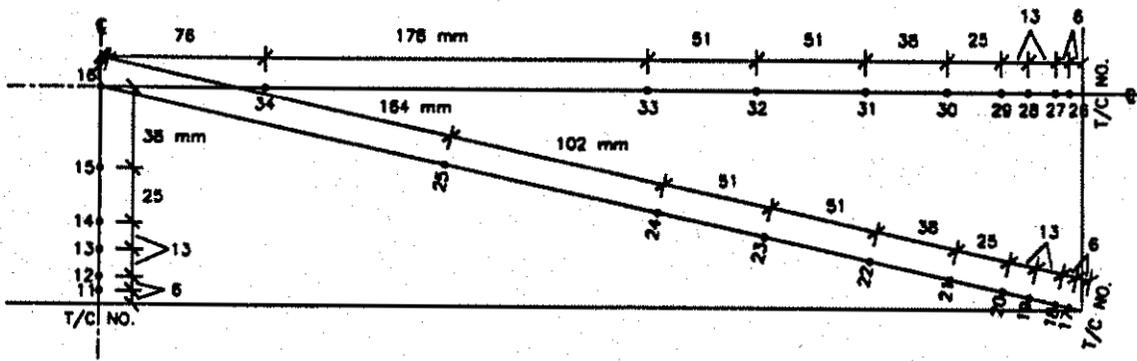
FIGURE 14 LOCATIONS OF T/C'S IN FRAMES: COLUMN NO. 4
