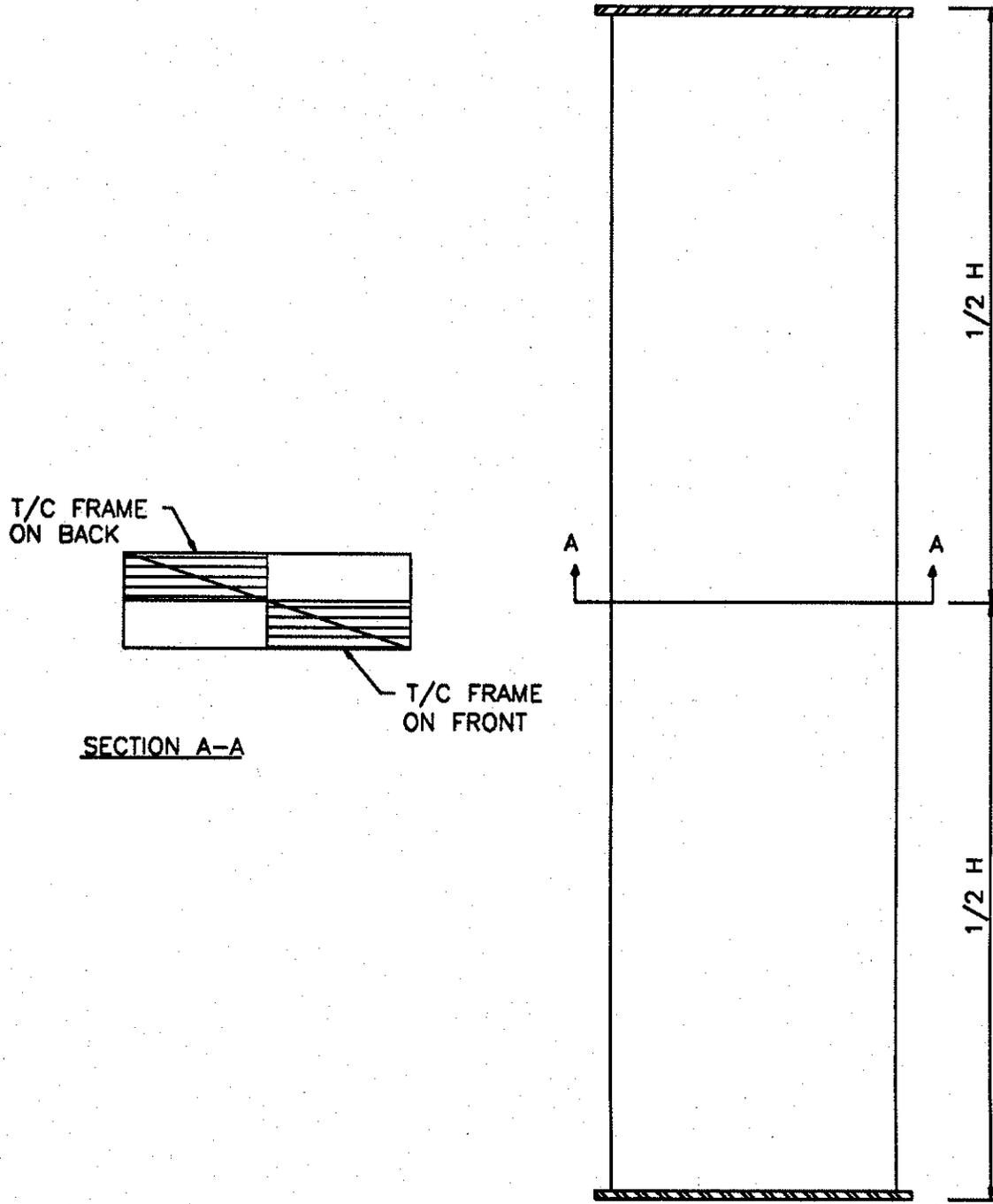
FIGURE 13 LAYOUT OF T/C FRAMES IN CONCRETE: COLUMN NO. 4 (203 x 914 mm)
