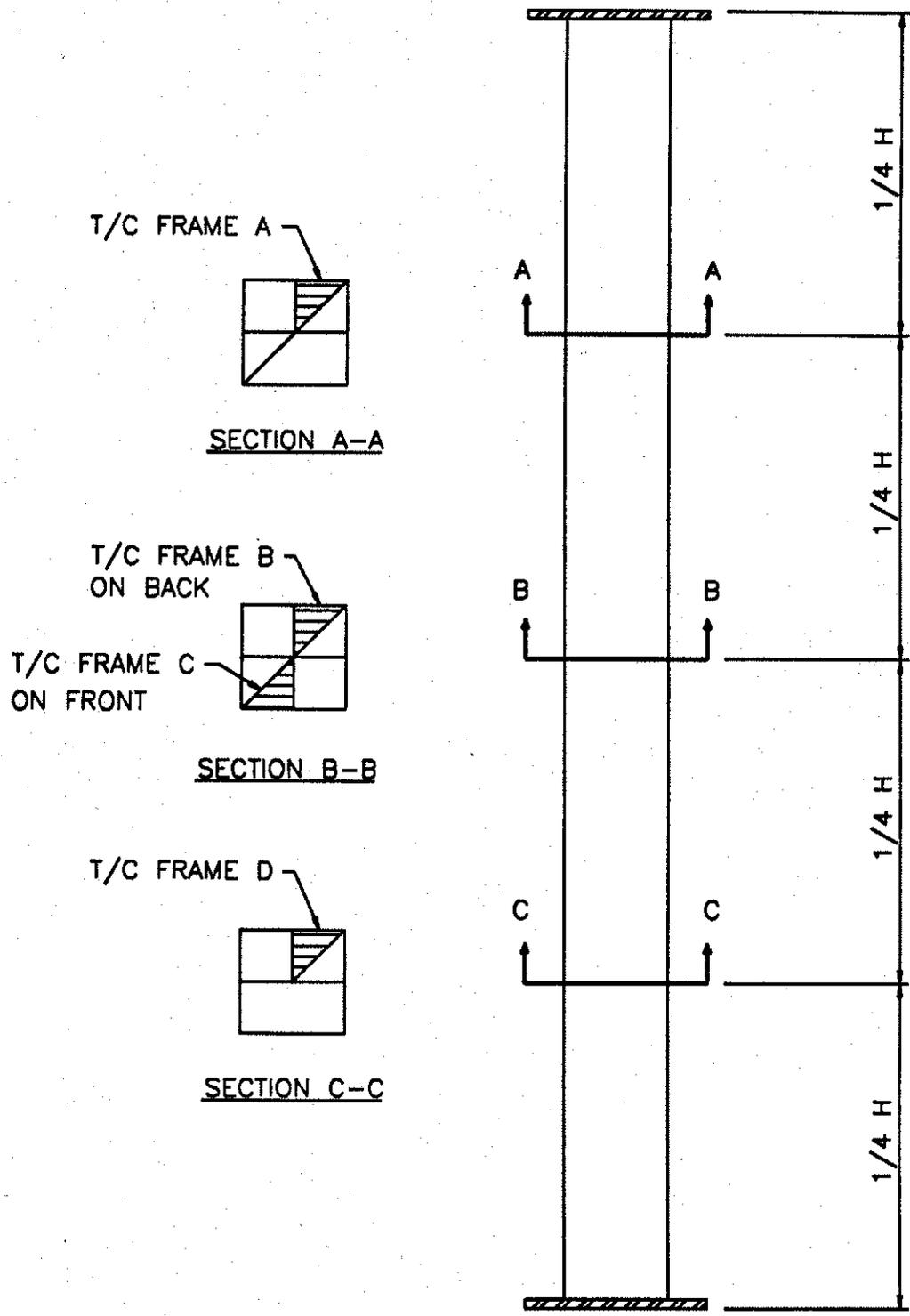
FIGURE 5 LAYOUT OF T/C FRAMES IN CONCRETE: COLUMN NO. 1 (305 x 305 mm, 4 BARS)
