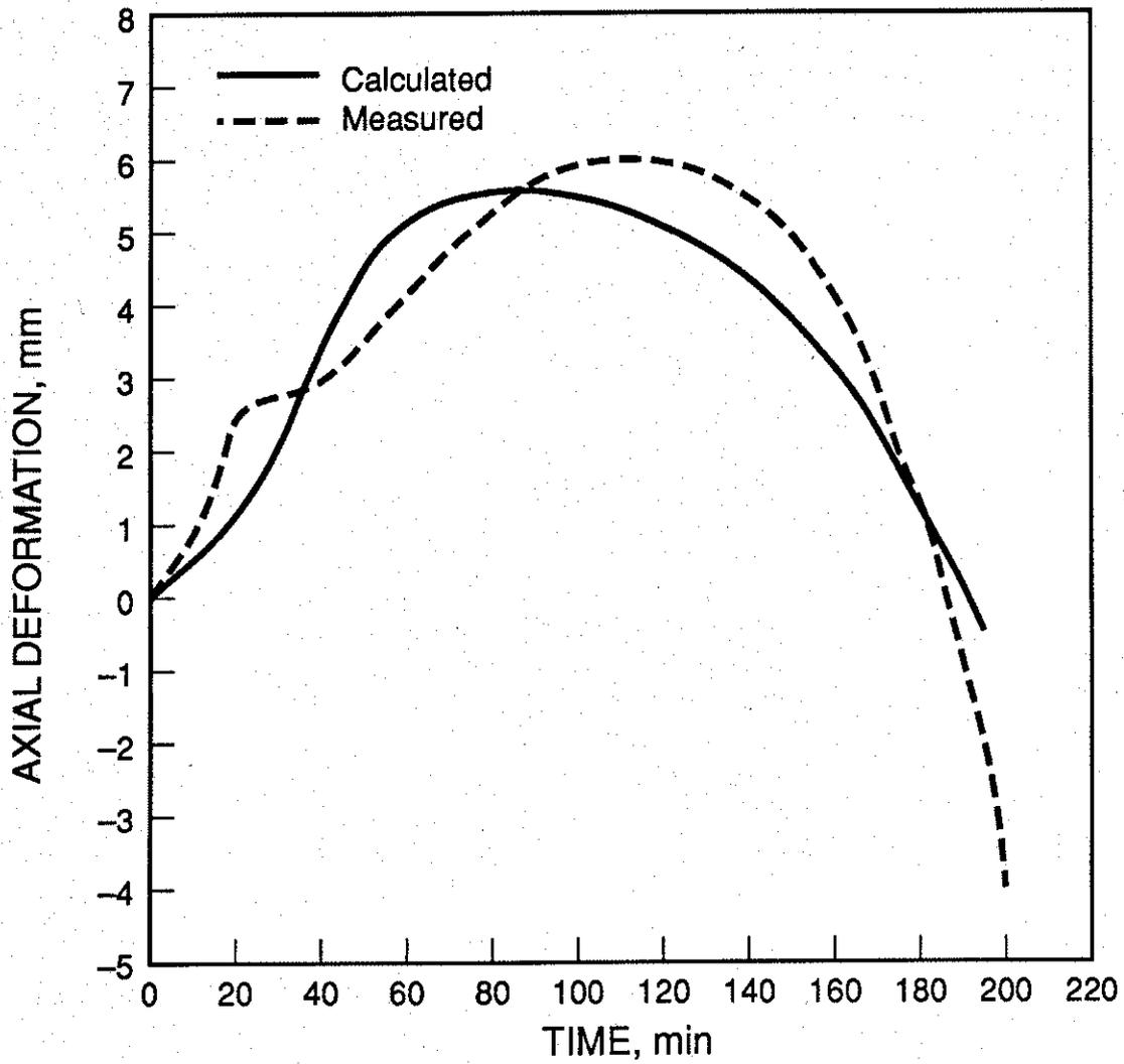
FIGURE 24. CALCULATED AND MEASURED AXIAL DEFORMATIONS OF COLUMN NO. 1 (305 x 305 mm, 4 BARS) AS A FUNCTION OF EXPOSURE TIME
