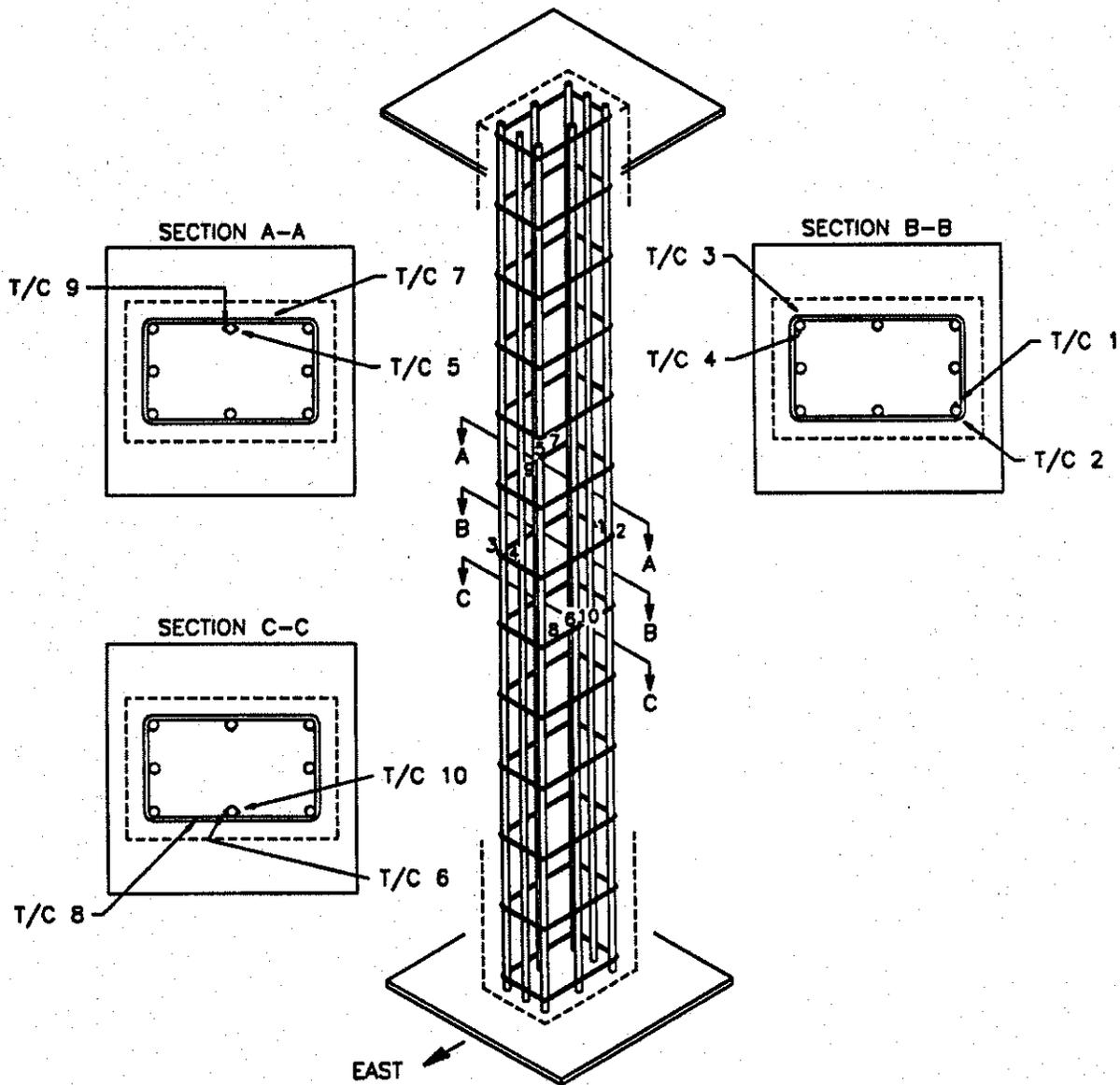
FIGURE 12 LOCATIONS OF T/C'S ON REINFORCING BARS:
