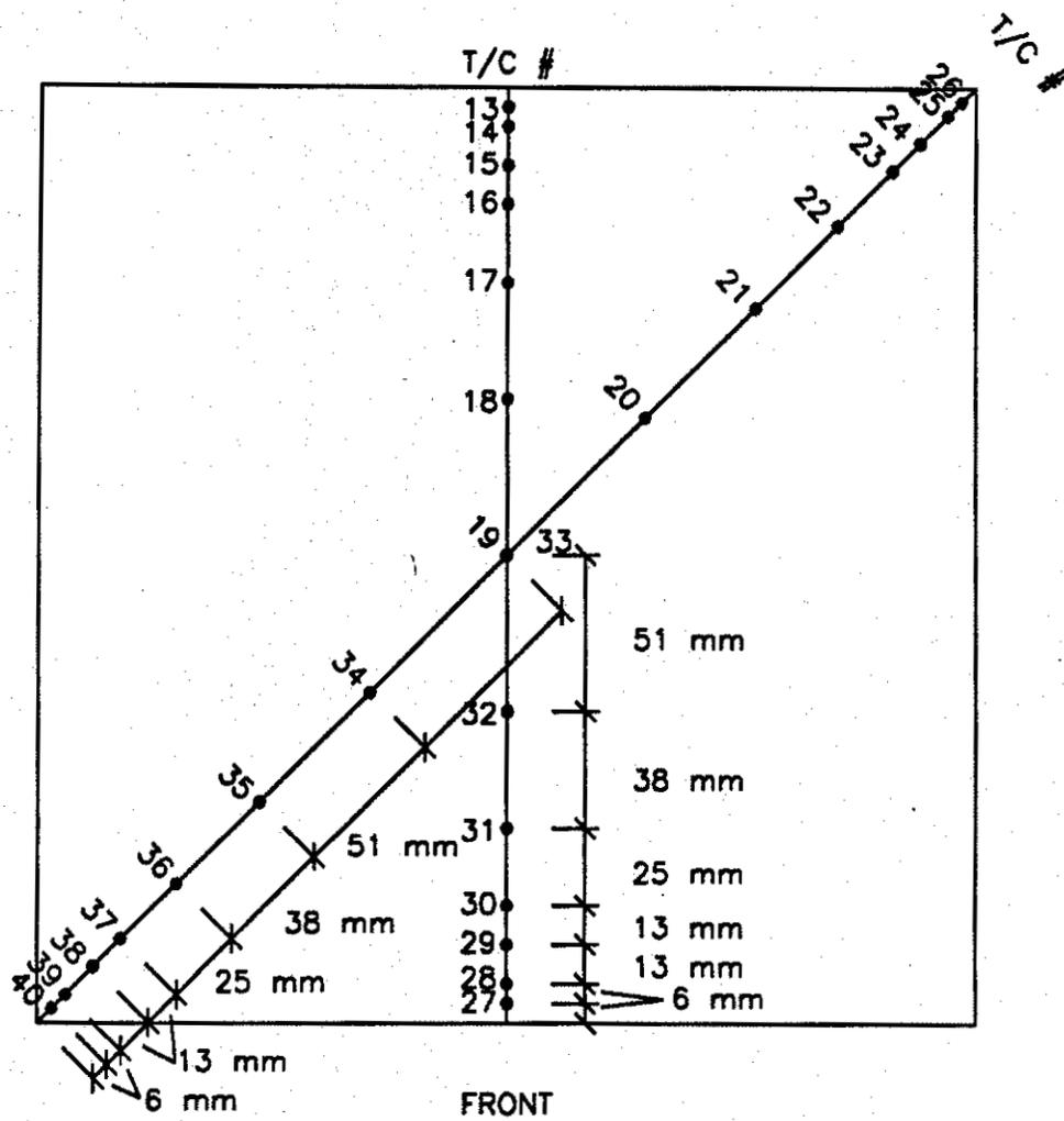
FIGURE 8 LOCATIONS OF T/C'S IN FRAMES: COLUMN NO. 2
