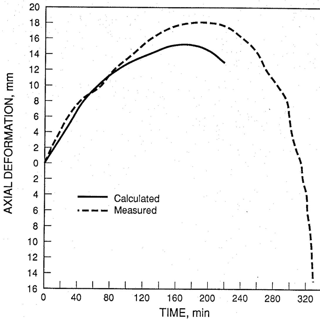
FIGURE 27. CALCULATED AND MEASURED AXIAL DEFORMATIONS OF COLUMN NO. 4 (203 x 914 mm) AS A FUNCTION OF EXPOSURE TIME
