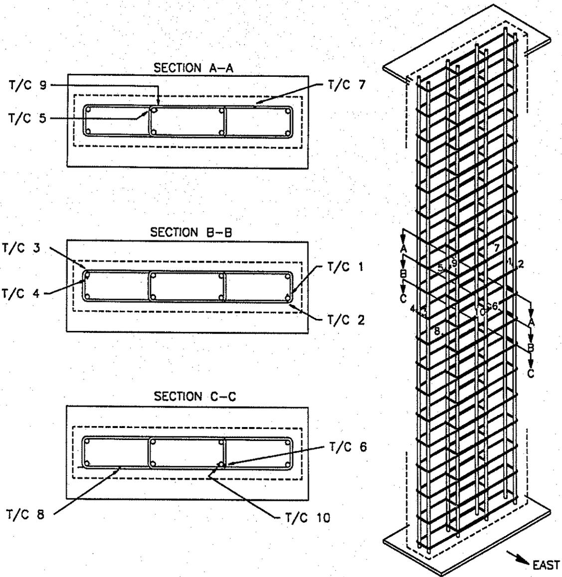
FIGURE 15 LOCATIONS OF T/C'S ON REINFORCING BARS:
