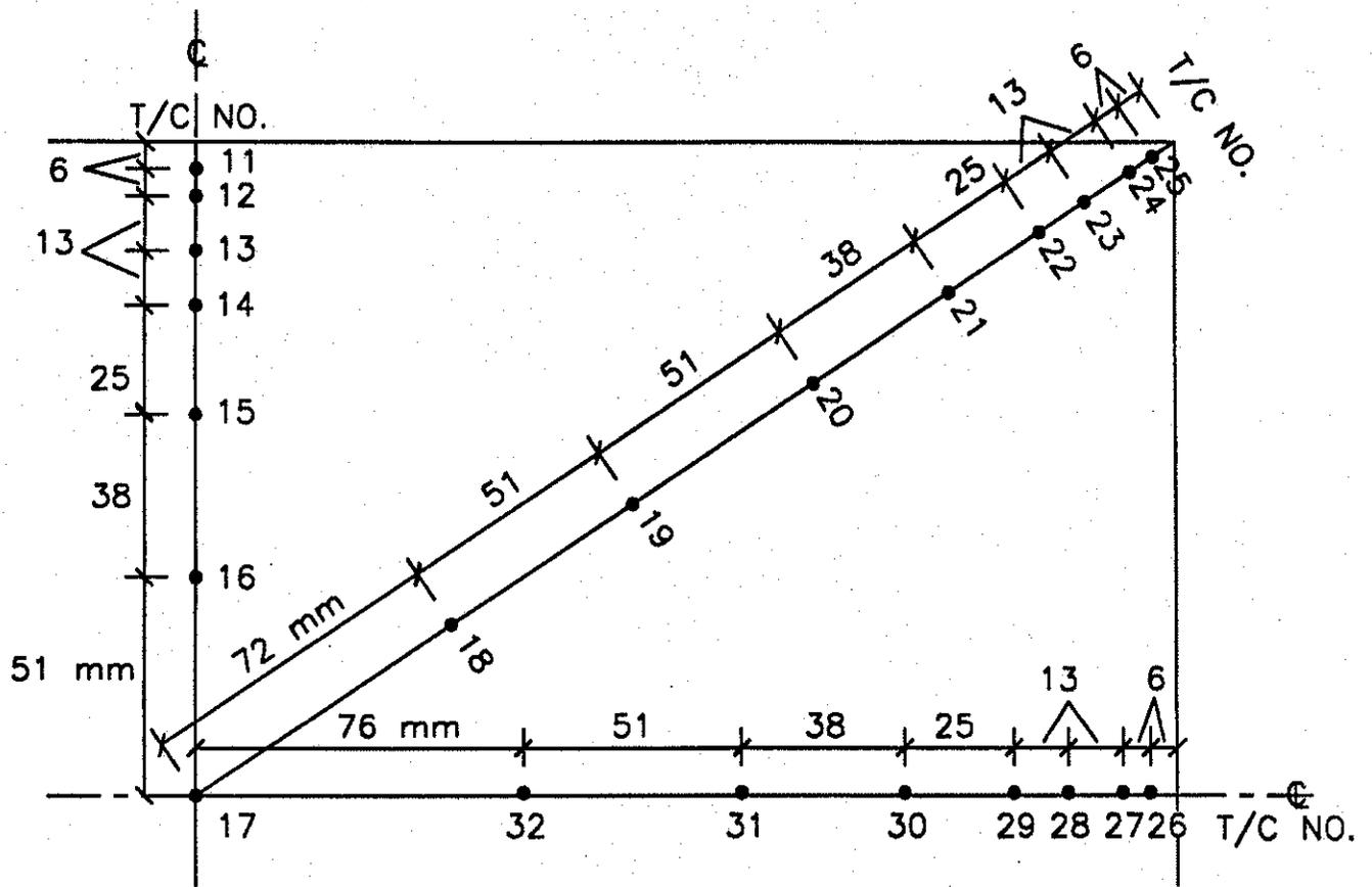
FIGURE 11 LOCATIONS OF T/C'S IN FRAMES: COLUMN NO. 3
