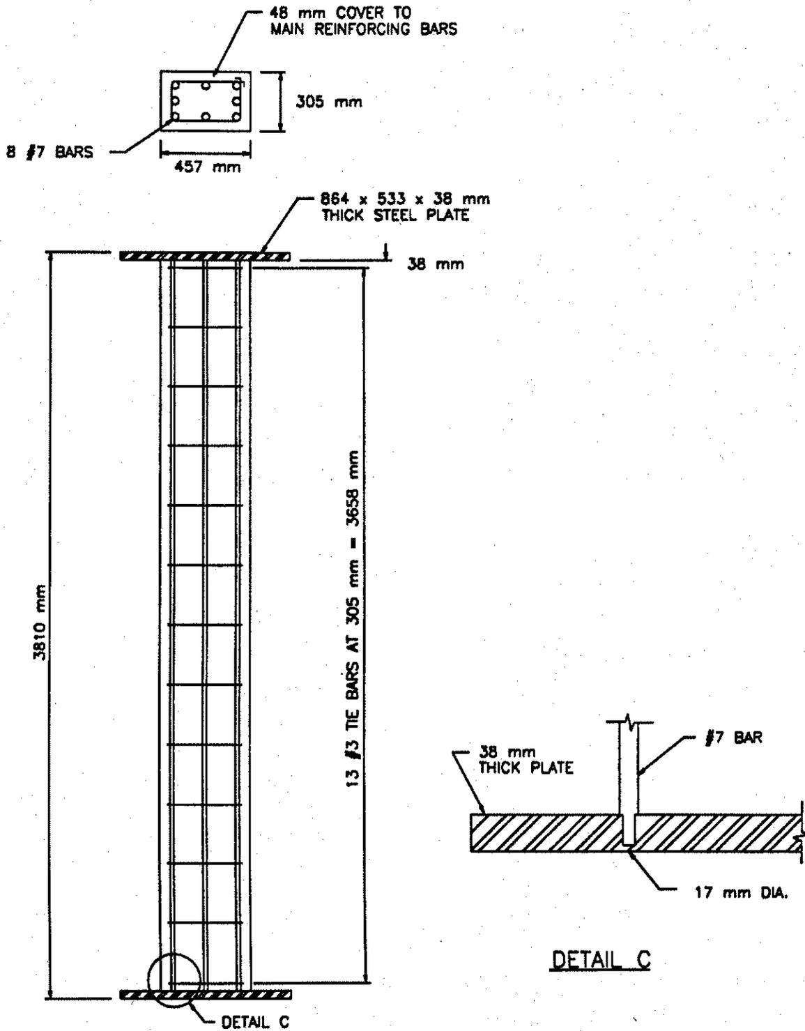
FIGURE 3 ELEVATION, CROSS-SECTION AND FINISHING DETAIL:
