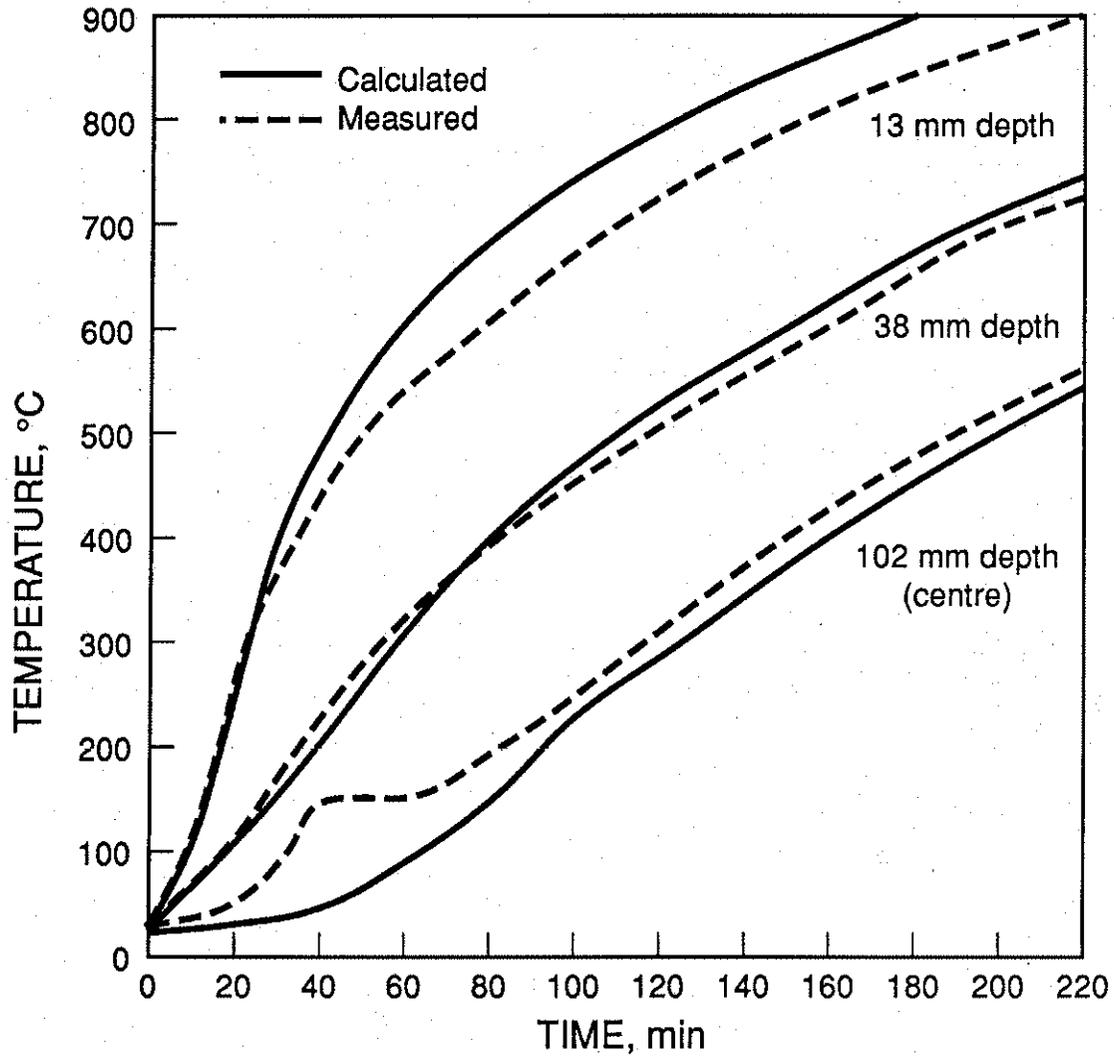
FIGURE 23. TEMPERATURES OF CONCRETE AT VARIOUS DEPTHS ALONG CENTRELINE PARALLEL TO SHORTEST SIDE OF COLUMN NO. 4 (203 x 914 mm) AS A FUNCTION OF EXPOSURE TIME
