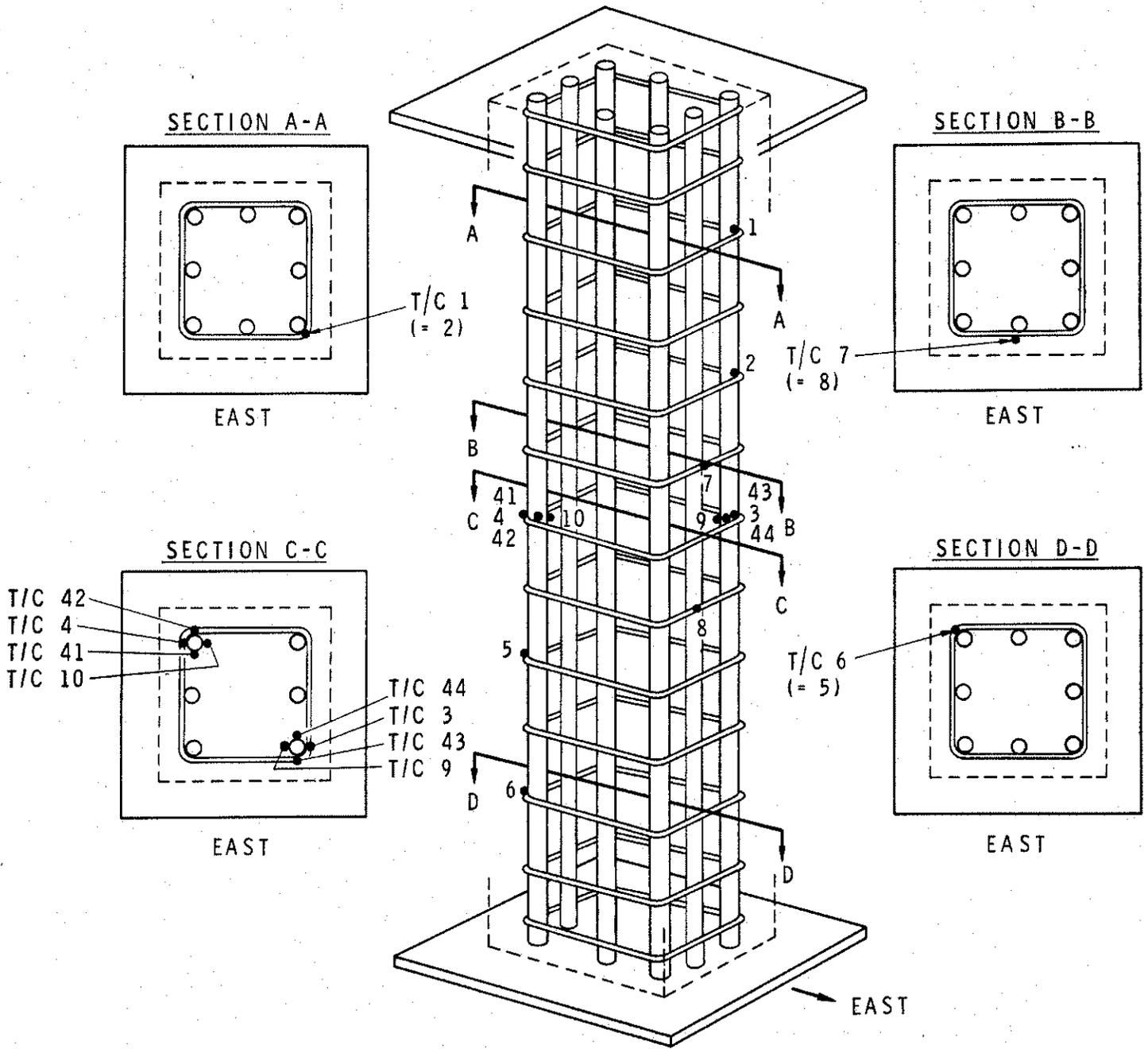
FIGURE 9 LOCATIONS OF T/C'S ON REINFORCING BARS:
