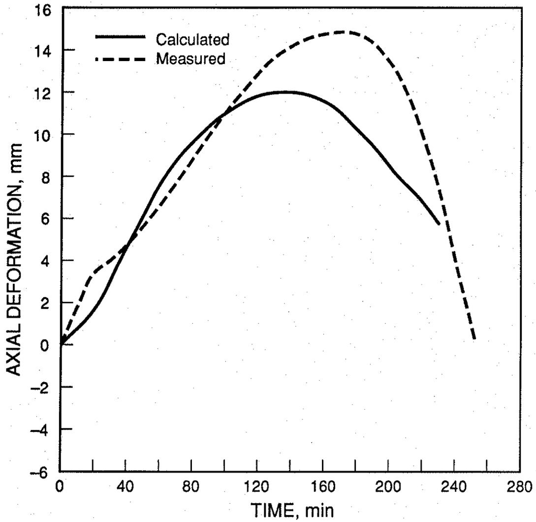
FIGURE 25. CALCULATED AND MEASURED AXIAL DEFORMATIONS OF COLUMN NO. 2 (305 x 305 mm, 8 BARS) AS A FUNCTION OF EXPOSURE TIME
