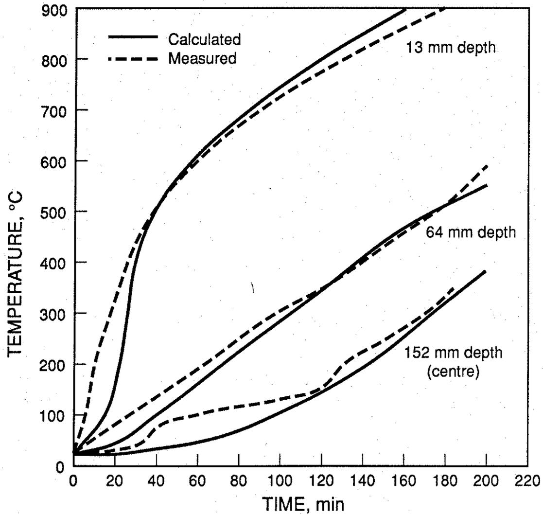
FIGURE 21. TEMPERATURES OF CONCRETE AT VARIOUS DEPTHS ALONG CENTRELINE OF SQUARE COLUMN NO. 1 (305 x 305 mm) AS A FUNCTION OF EXPOSURE TIME
