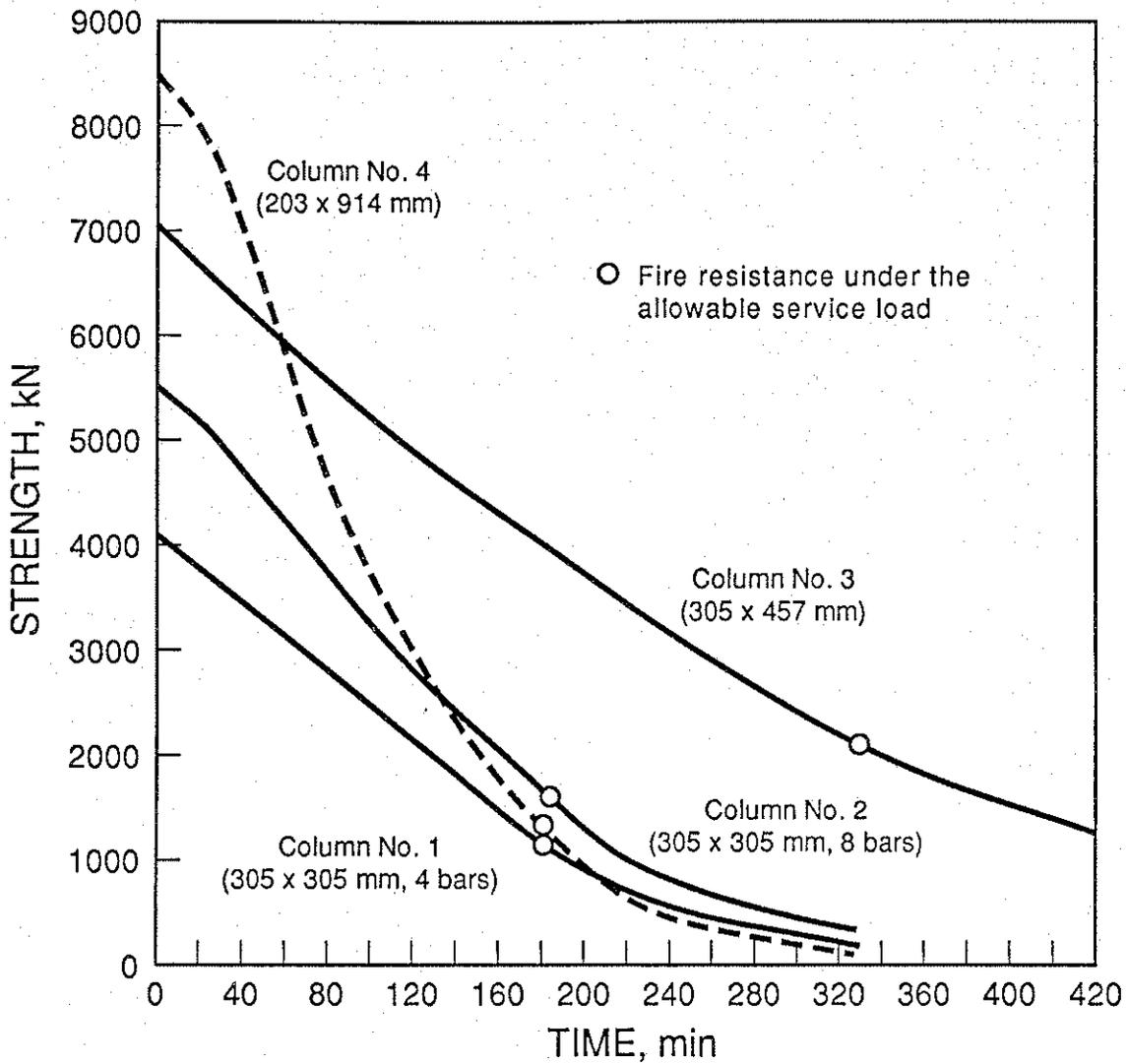
FIGURE 28. CALCULATED STRENGTHS OF COLUMNS AS A FUNCTION OF EXPOSURE TIME AND CALCULATED COLUMN FIRE RESISTANCES UNDER THE ALLOWABLE SERVICE LOAD ACCORDING TO ACI 318-89 AND CSA A23.3-M84
