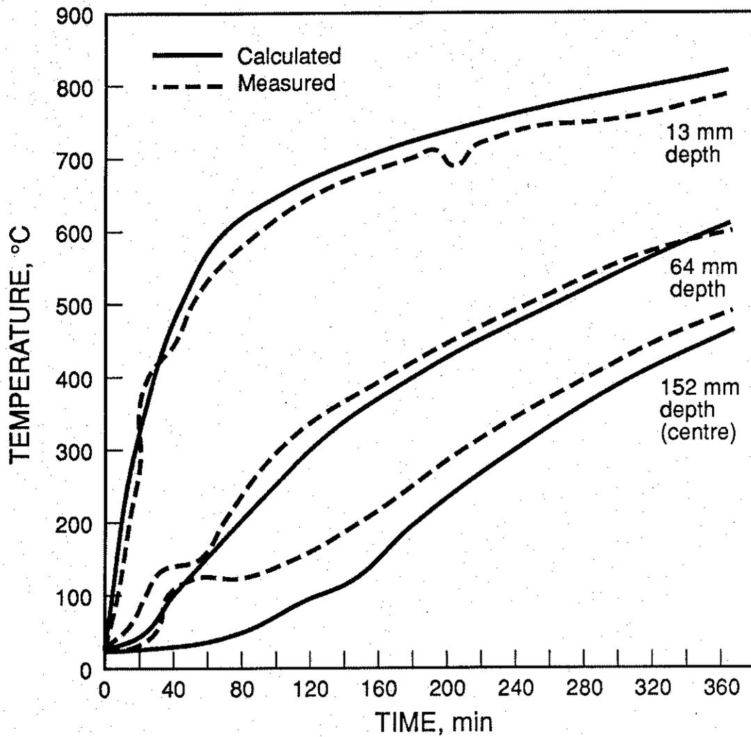
FIGURE 22. TEMPERATURES OF CONCRETE AT VARIOUS DEPTHS ALONG CENTRELINE PARALLEL TO SHORTEST SIDE OF COLUMN NO. 3 (305 x 457 mm) AS A FUNCTION OF EXPOSURE TIME
