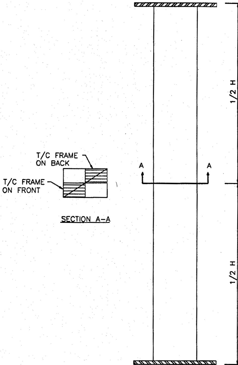
FIGURE 10 LAYOUT OF T/C FRAMES IN CONCRETE: COLUMN NO. 3 (305 x 457 mm)
