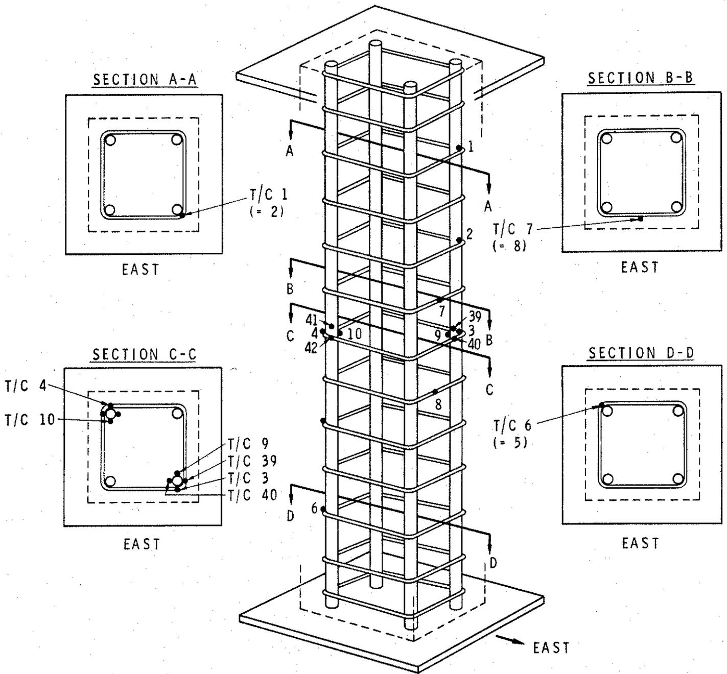
FIGURE 7 LOCATIONS OF T/C'S ON REINFORCING BARS:
