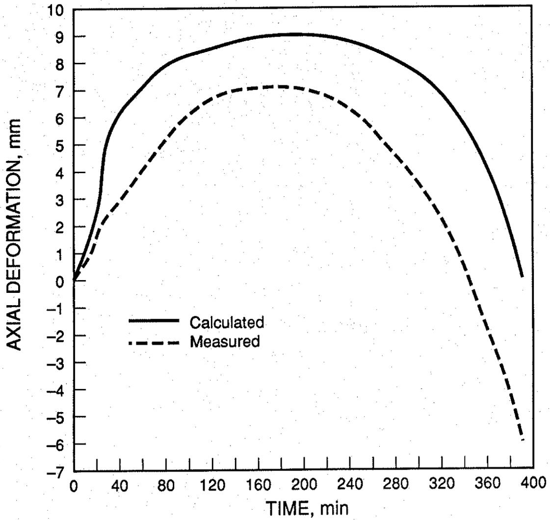
FIGURE 26. CALCULATED AND MEASURED AXIAL DEFORMATIONS OF COLUMN NO. 3 (305 x 457 mm) AS A FUNCTION OF EXPOSURE TIME
