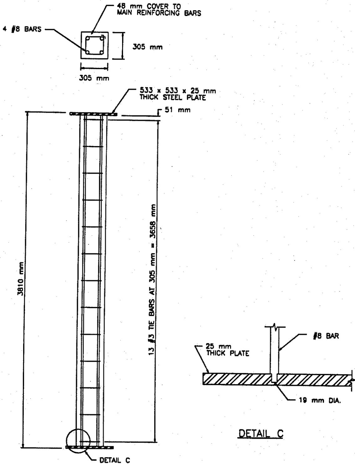
FIGURE 1 ELEVATION, CROSS-SECTION AND FINISHING DETAIL:
