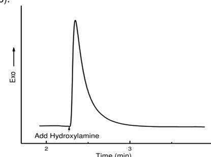
Figure 2. DSC trace of the reactive silver ink at room temperature when hydroxylamine was added.
