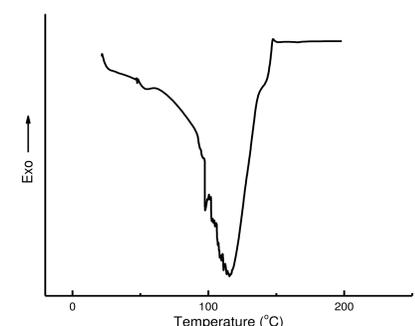
Figure 3. DSC trace of the reactive silver ink during its heating process.
