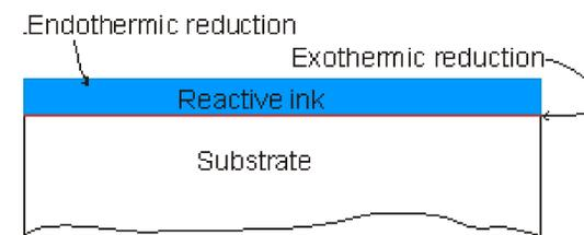
Figure 1. The design of a silver deposition process that doesn't need external heat
