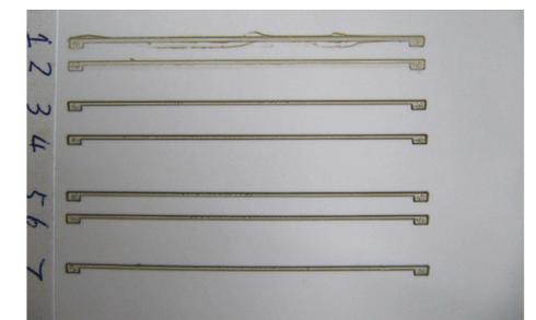
Figure 6. Silver lines printed using inkjet printer on Canon photo paper. Printed at room temperature and without any post treatment.
