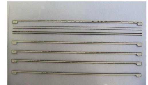
Figure 5. Silver lines printed using inkjet printer on PET film. Printed at room temperature and without any post treatment
