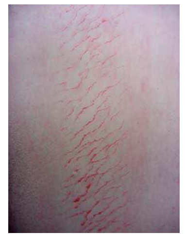
B) Micro-cracks on the field/rim side of the high-speed wheel.
