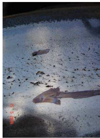
D) Well-defined cracks on the field/rim side of the wheel.
