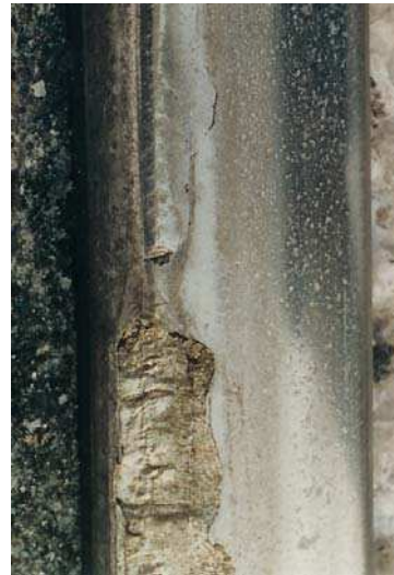
B) gauge-corner collapse in a well-lubricated rail
