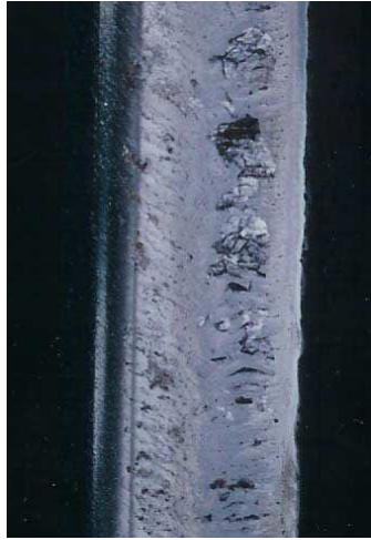
G) Alternating wet/dry conditions → shallow shelling.
