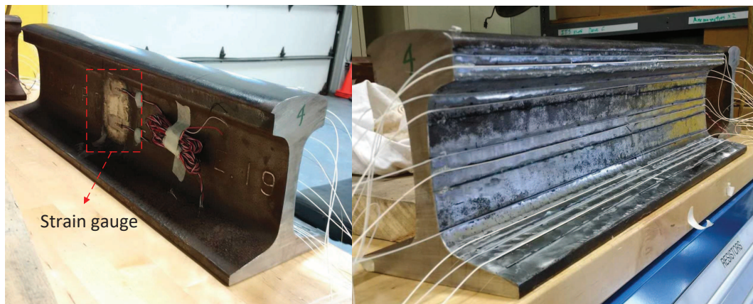
Figure 1. Rail specimen instrumented with strain gauge and optical fibers on each side.
