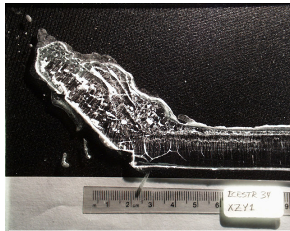
Figure 2: A typical cross-section of a sample collected in Test ICESTR34: 12-mm thick freshwater ice (side of cone).
