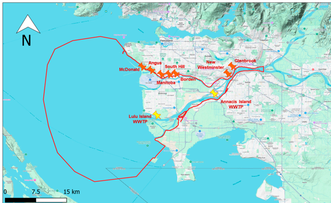
Figure 3. Locations of CSOs (orange pins) and WWTPs (yellow pins), representing release sources of microplastic particles.
