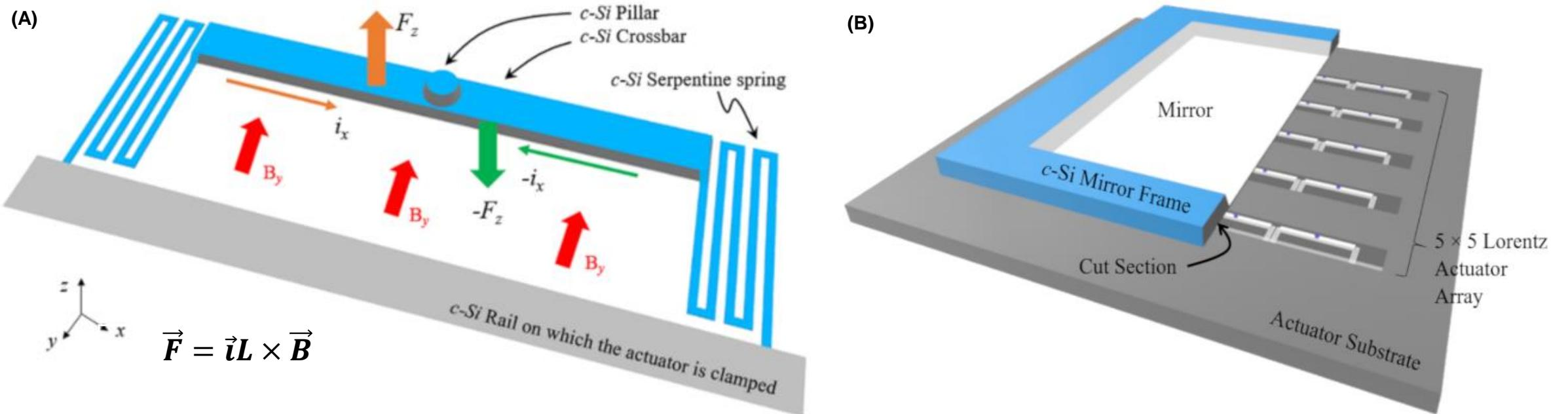
Figure. Illustration of a Lorentz force actuator showing the working principle (A), and a  $5 \times 5$  array of Lorentz actuators with mirror attached (B)
