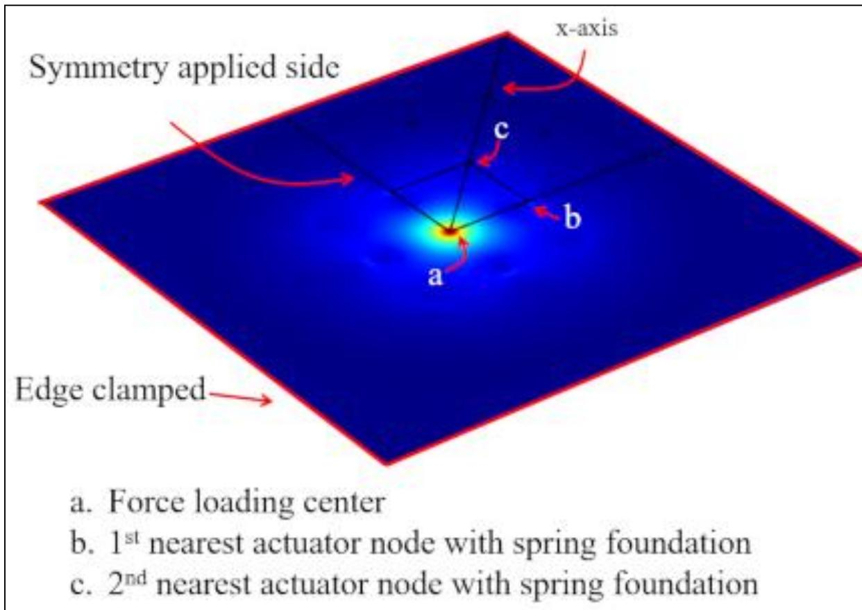
STEP 1: Simulation on inter-actuator coupling and corresponding actuator spring constant with 5 x 5 actuator array (spring foundation)
