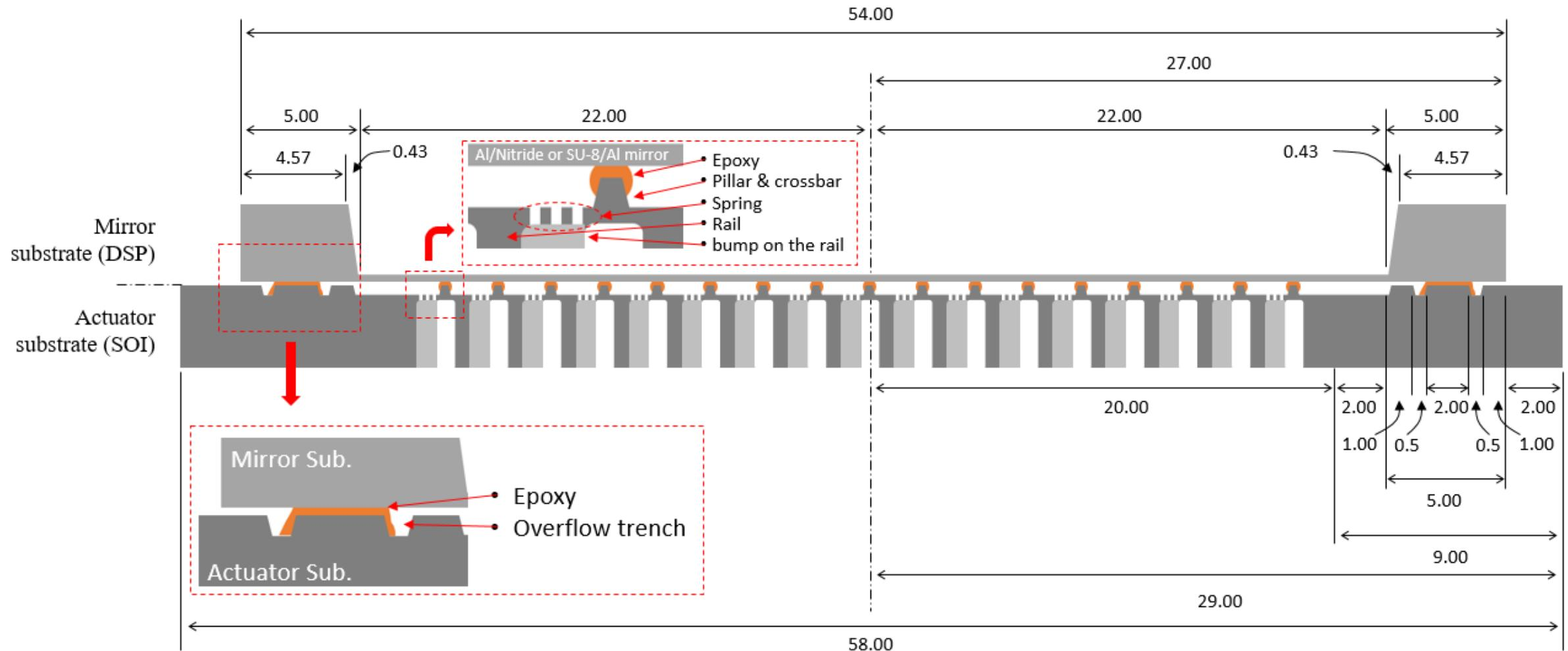
System can be represented by thin membrane mirror with an array of spring attached
