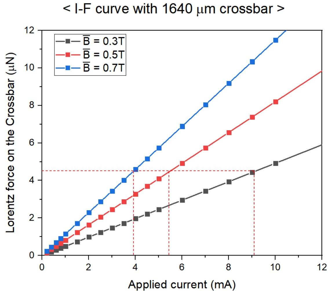
Figure: operation current in different magnetic field computed by  $\vec{F} = \vec{I}L \times \vec{B}$
