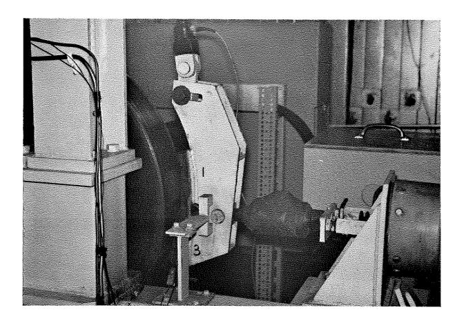
Fig. 8 Brake Shoe Carrier and Load Cells
