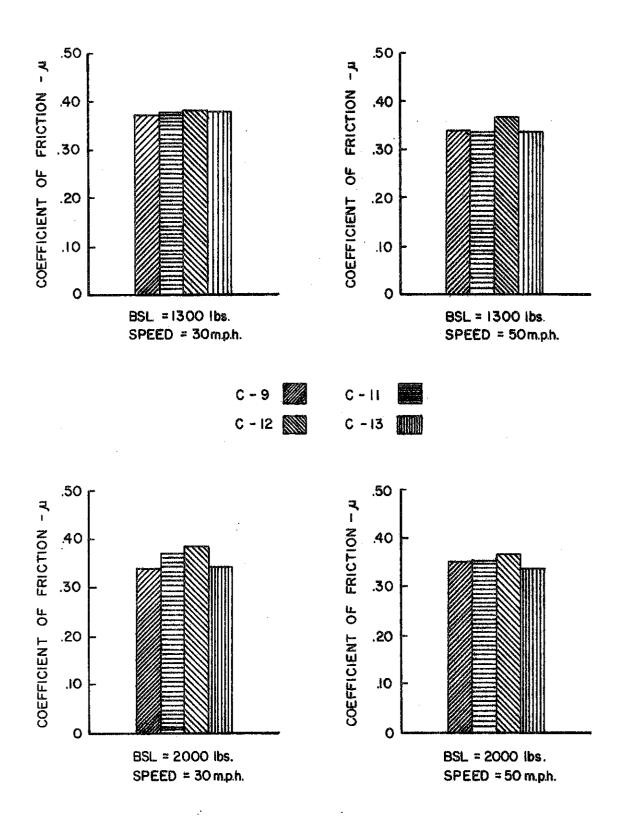
FIG. I COMPARISON OF FRICTION COEFFICIENTS - DRY TESTS
