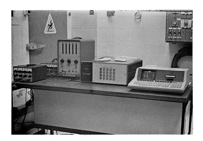
Fig. 11 Computerized Data Acquisition System
