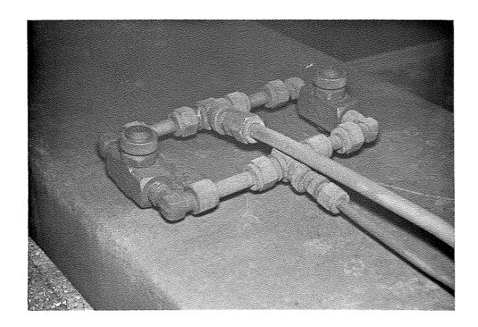
Fig. 9 Water Atomizing Nozzles
